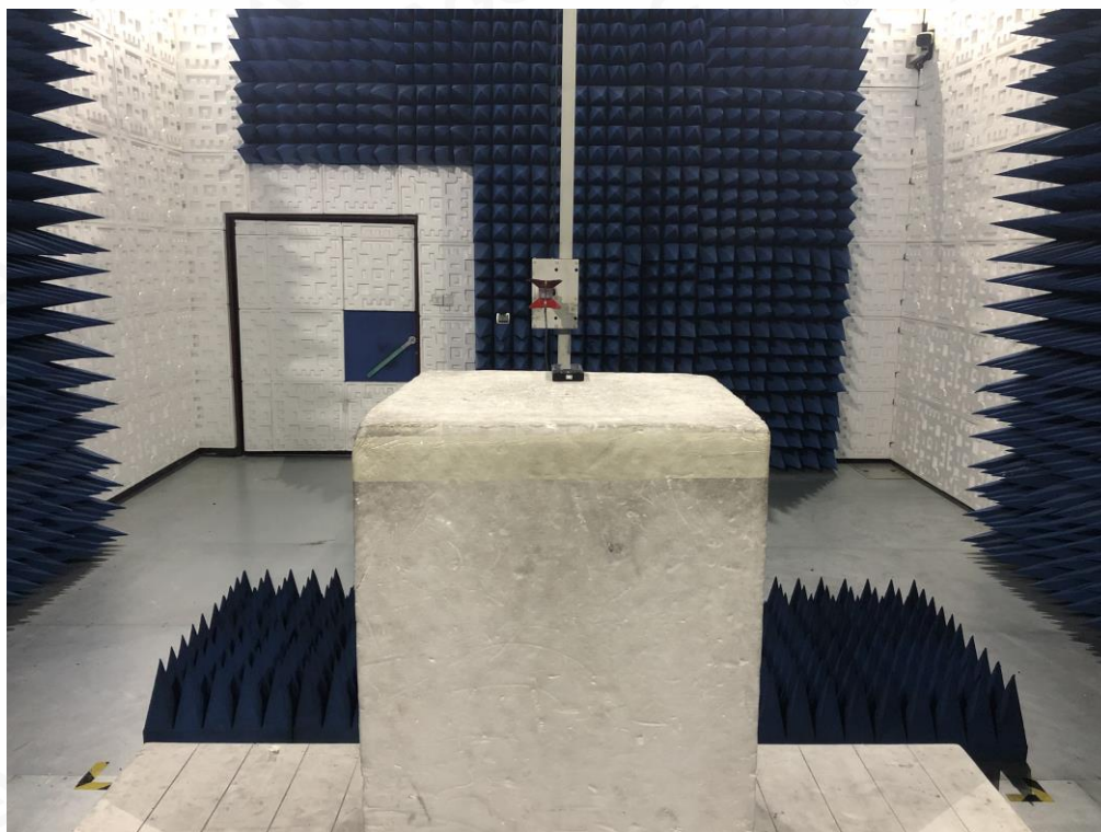
FCC RADIATED EMISSION TEST SETUP ABOVE 1GHZ
