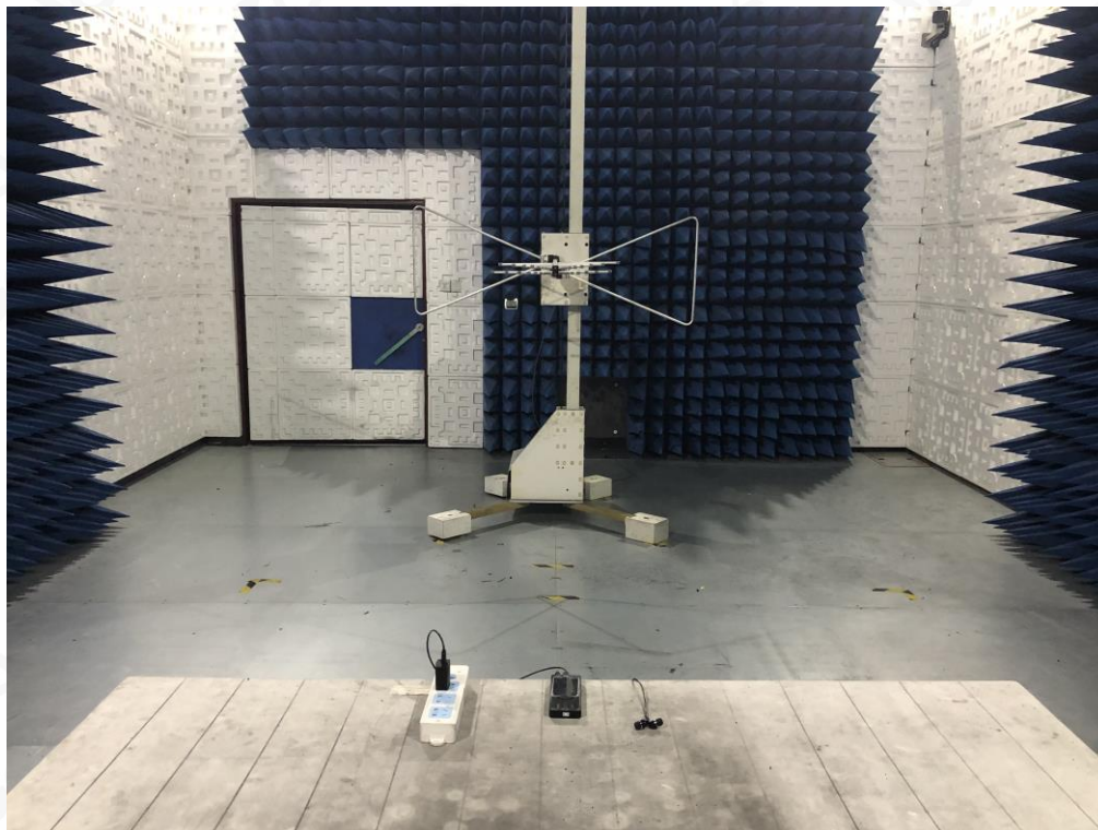
FCC RADIATED EMISSION TEST SETUP ABOVE 1GHZ
