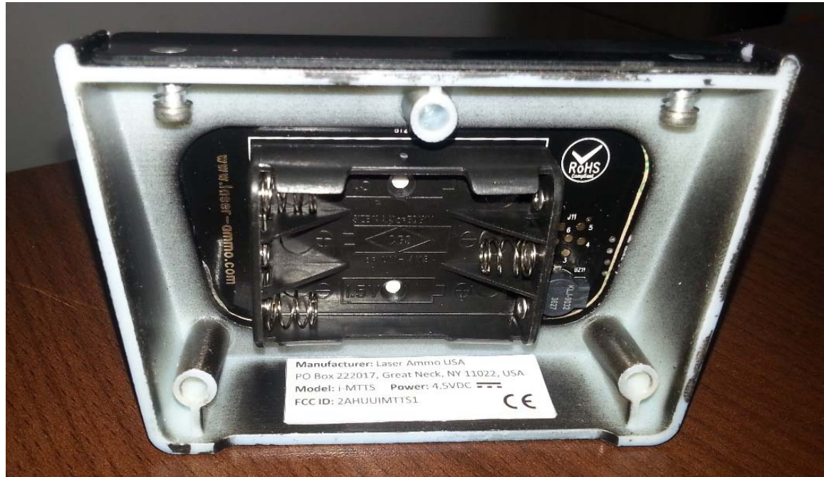
Photograph No.1 i-MTTS unit internal view
