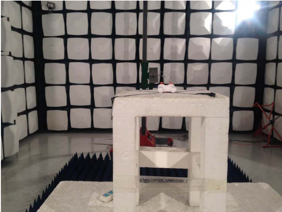
Photograph 3: Radiated Emission Test Configuration, (Above 1GHz) Front
