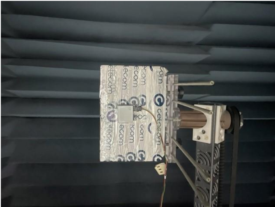
Photograph 3: EUT test setup in the FAC-2, EUT elevation 90°_below 12.4GHz
