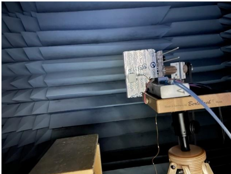
Photograph 2: EUT test setup in the FAC-2, EUT elevation 90°_overview
