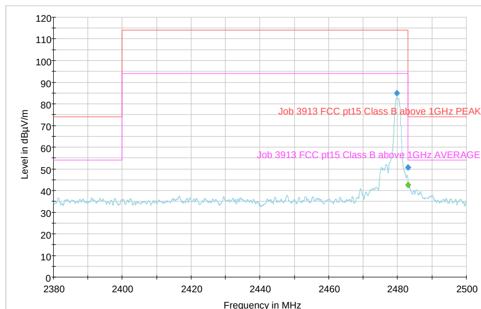
Transmit Power and Band Edge, Top Channel, X-Axis 2480MHz
