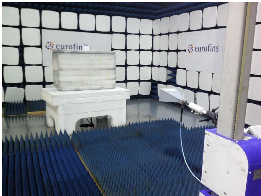
Radiated Emissions; Above 1 GHz
