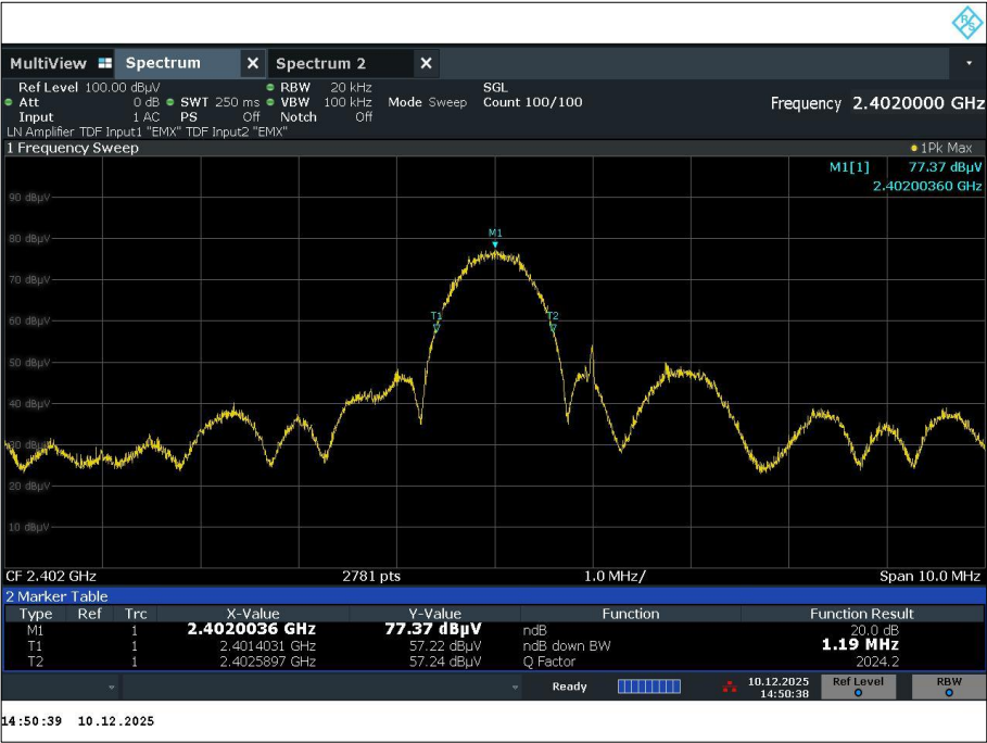
Figure 43 – CH37, 2402 MHz, 20 dB Bandwidth
