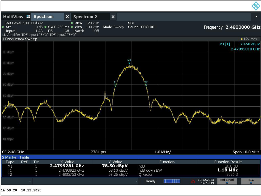
Figure 45 – CH39, 2480 MHz, 20 dB Bandwidth
