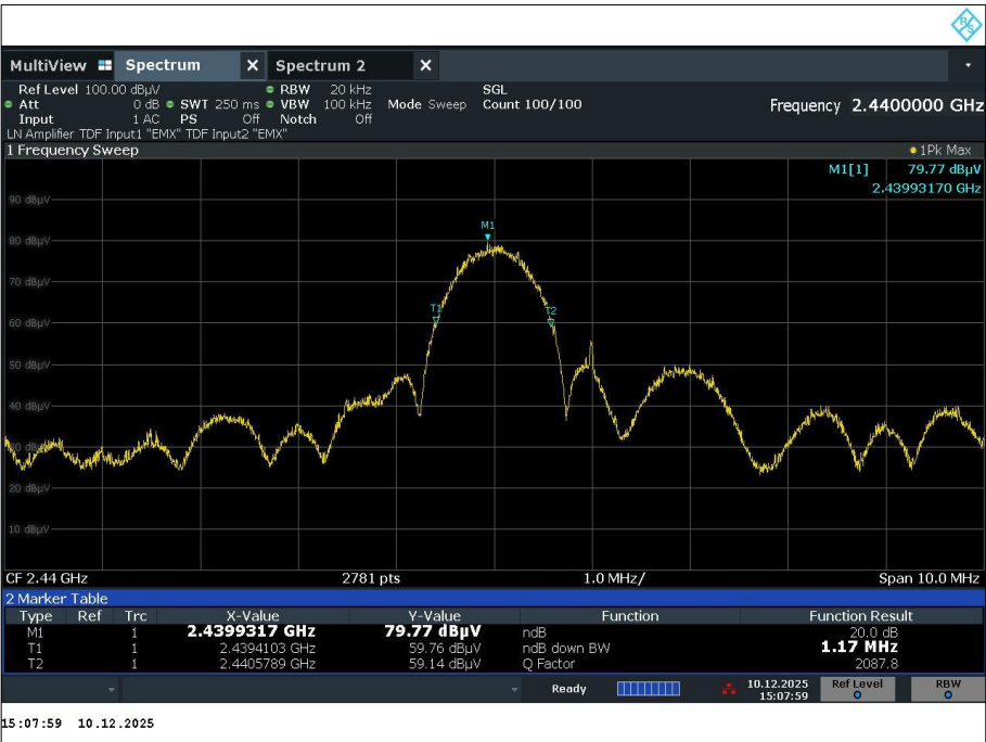
Figure 44 – CH19, 2440 MHz, 20 dB Bandwidth
