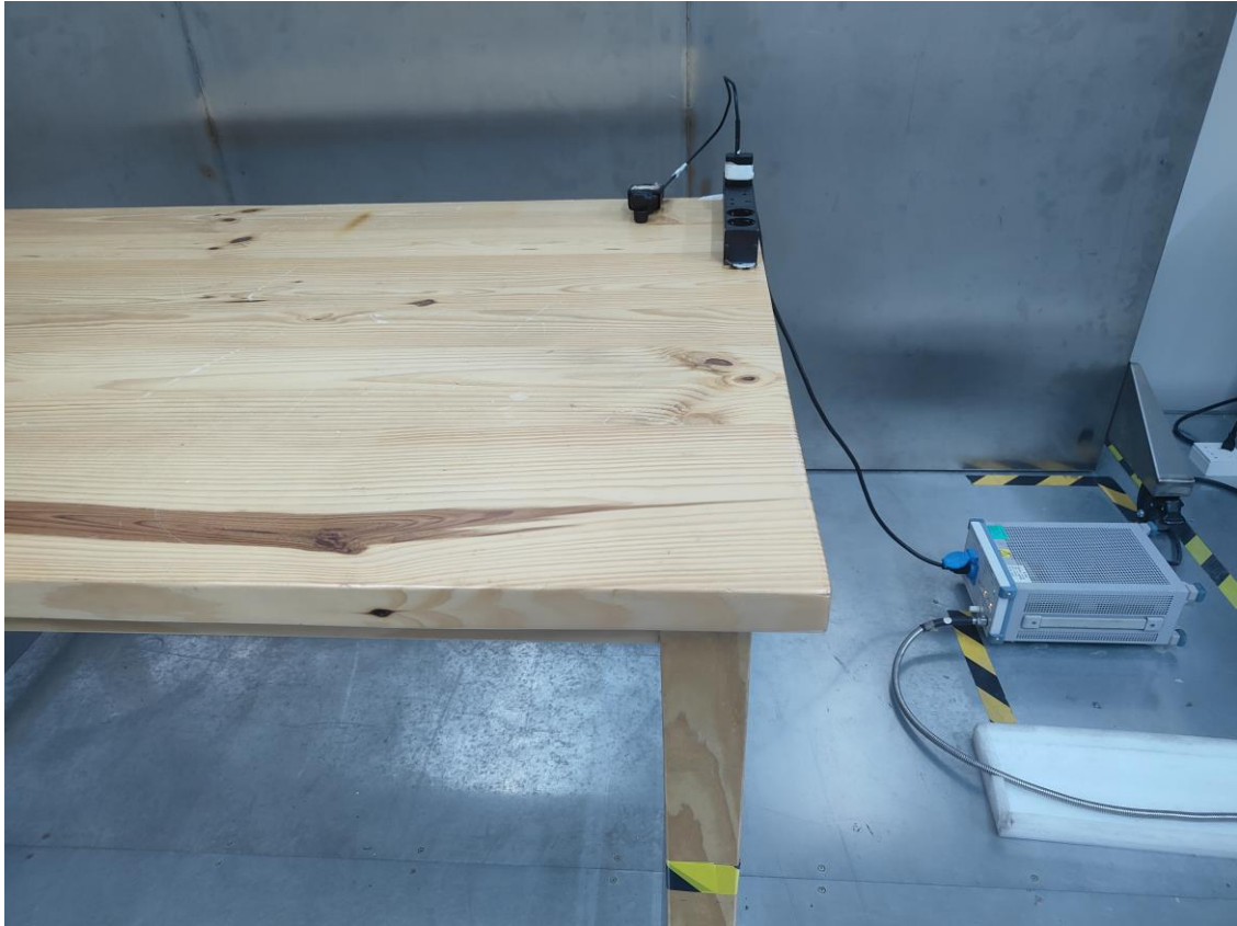
Conducted Emissions Side View
