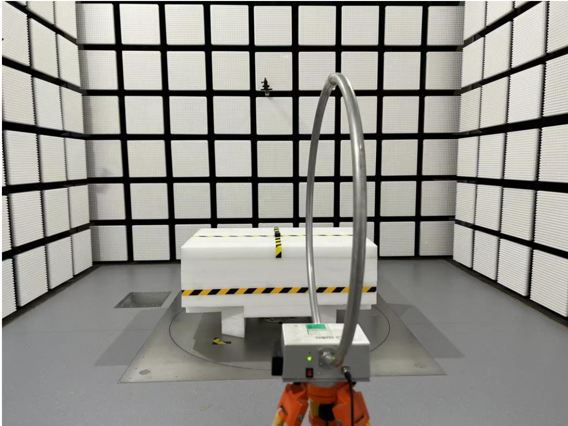
Radiated Emission 9 kHz-30 MHz Ground-parallel View
