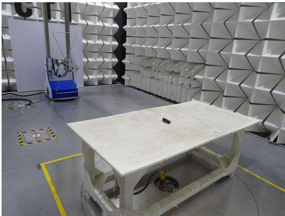
Radiated spurious emission Test Setup-2(Below 1GHz)
