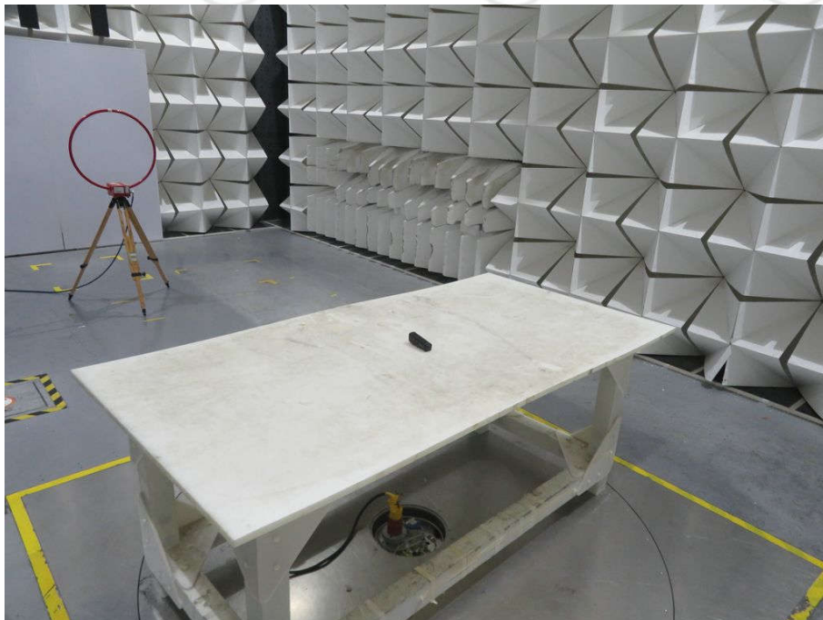
Radiated spurious emission Test Setup-1(Below 30MHz)
