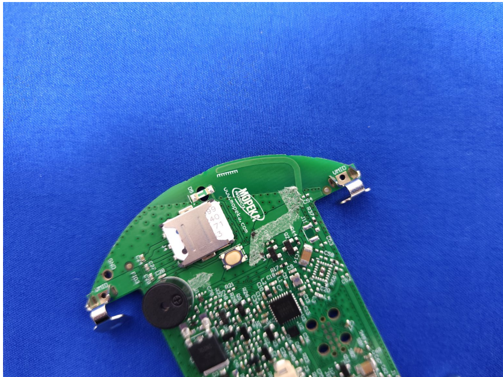
(12) EUT Photo(Antenna for BLE)
