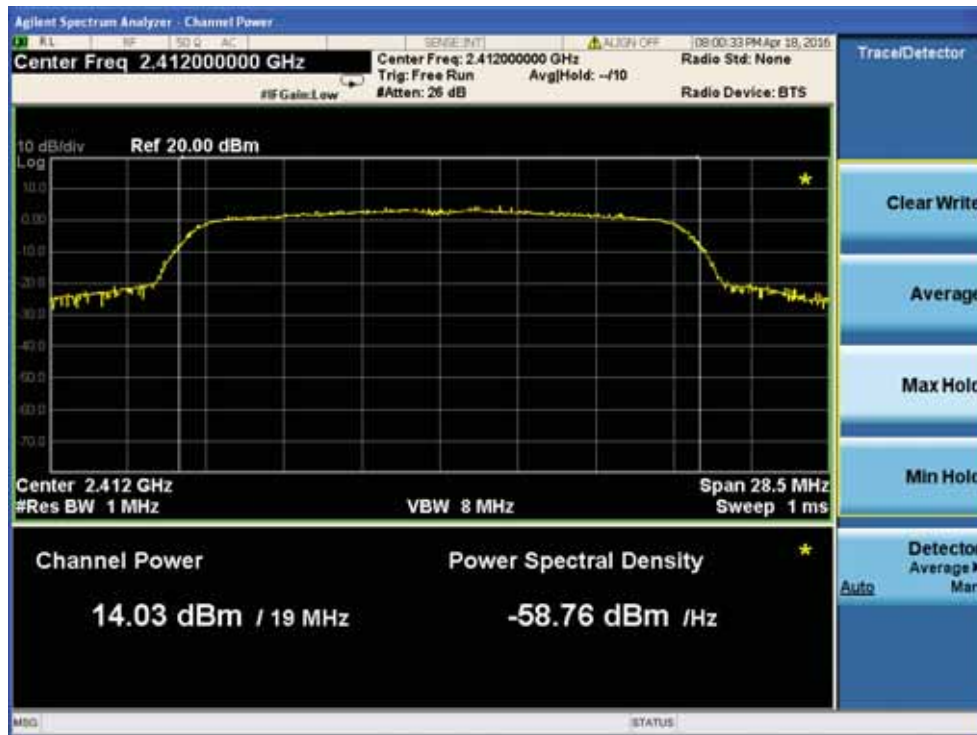
Output Power plot on channel 6
