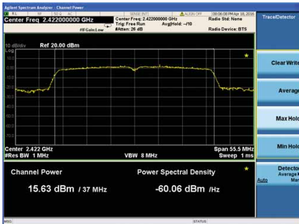
Output Power plot on channel 3
