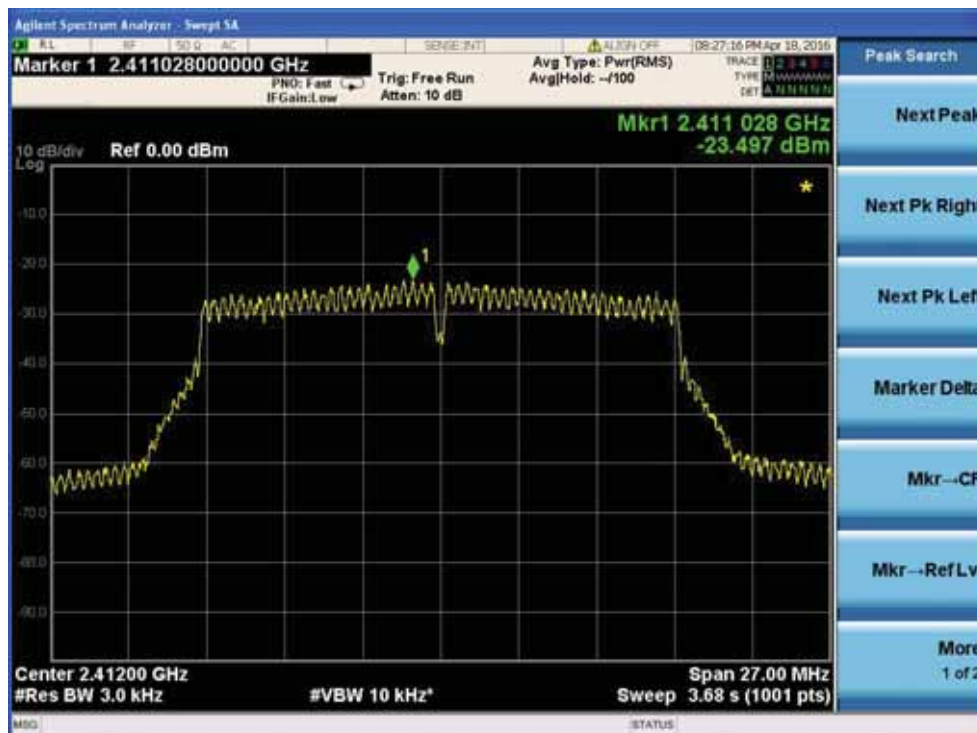
Power spectral density plot on channel 1
