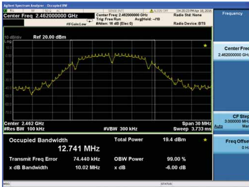
6dB Bandwidth plot on channel 1
