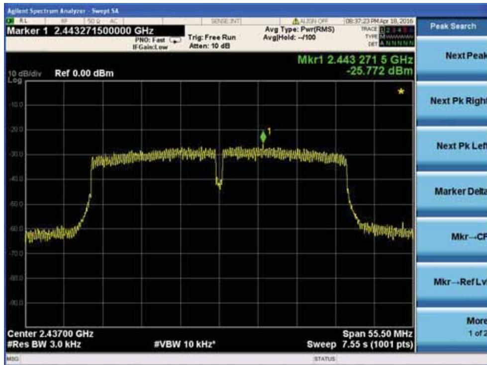
Power spectral density plot on channel 9
