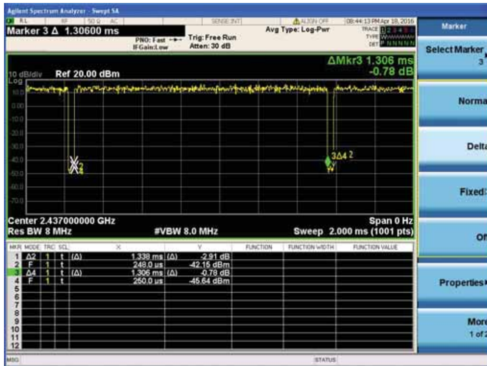
Duty Cycle plot on channel 6
