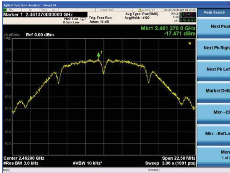
Power spectral density plot on channel 1
