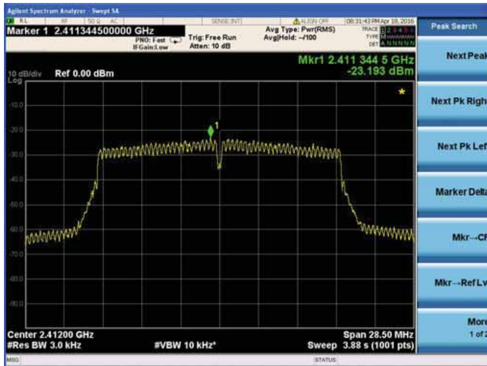
Power spectral density plot on channel 6
