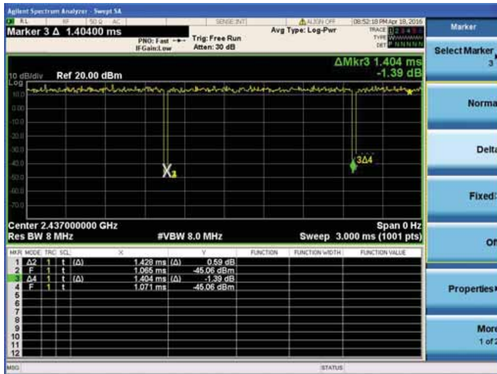
Duty Cycle plot on channel 6
