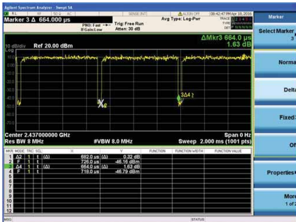
Duty Cycle plot on channel 6
