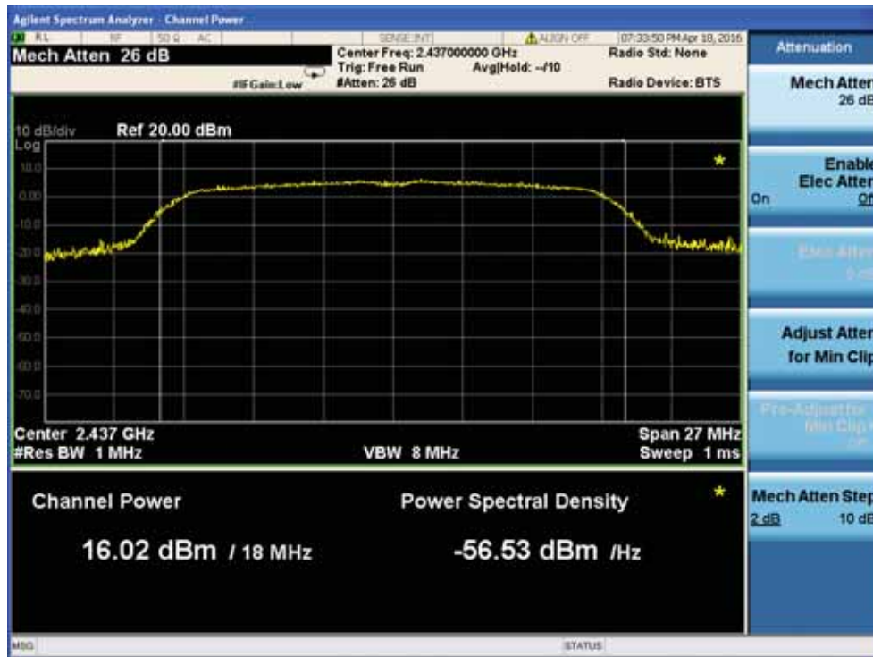
Output Power plot on channel 11
