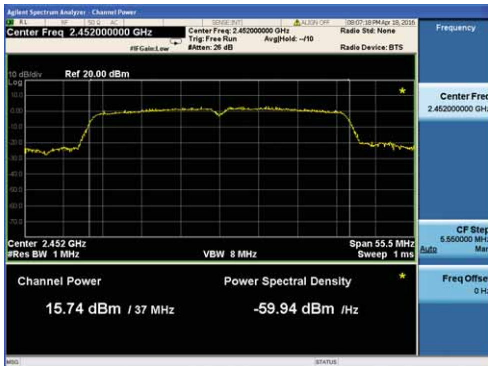
Output Power plot on channel 9
