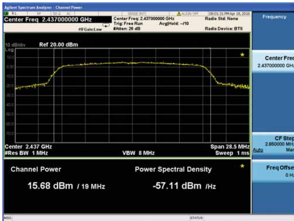
Output Power plot on channel 6
