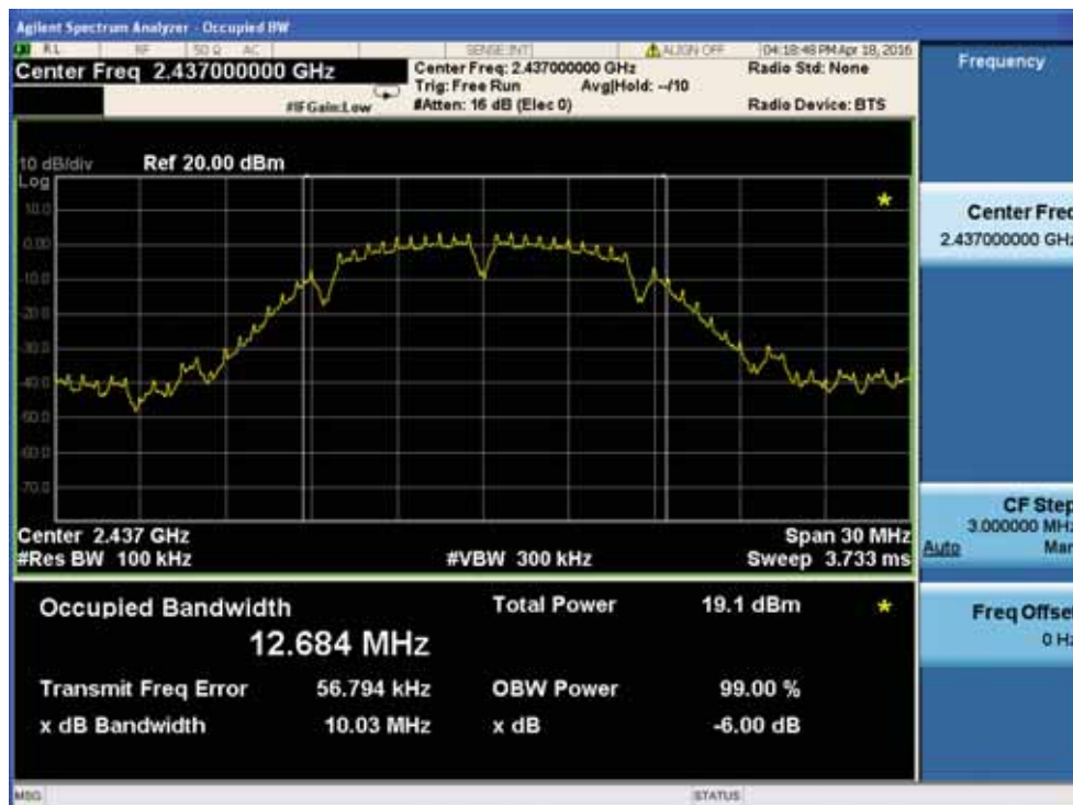
6dB Bandwidth plot on channel 6
