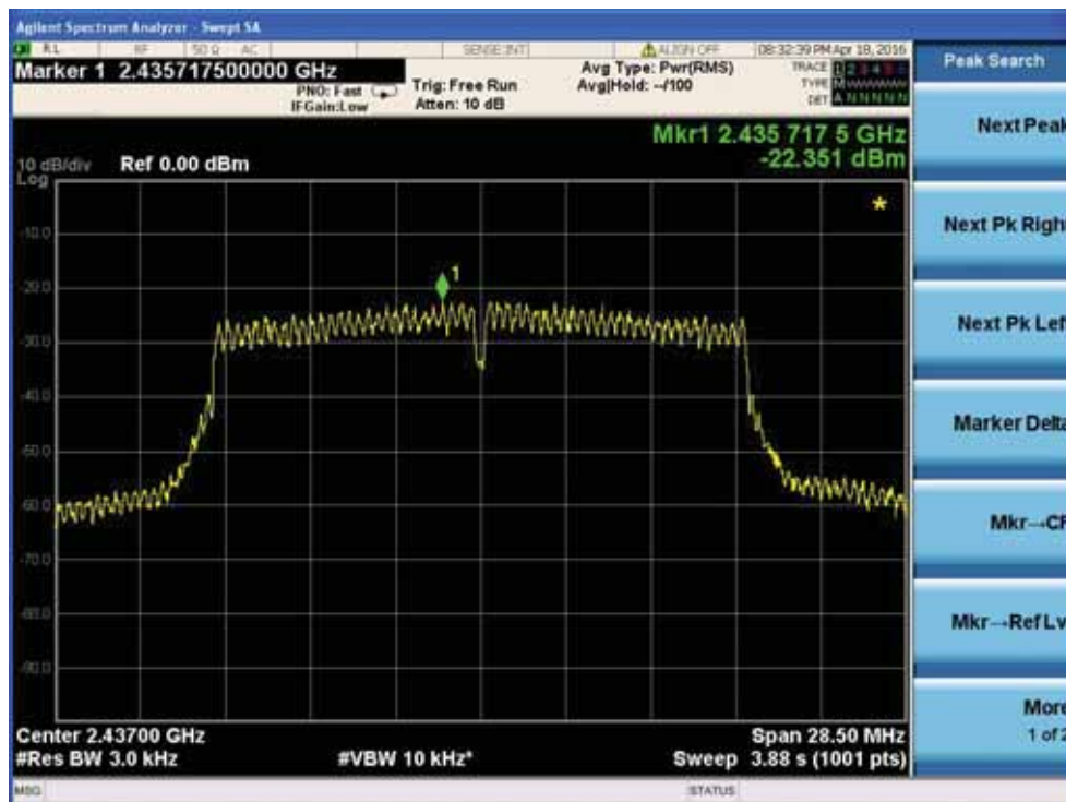
Power spectral density plot on channel 6
