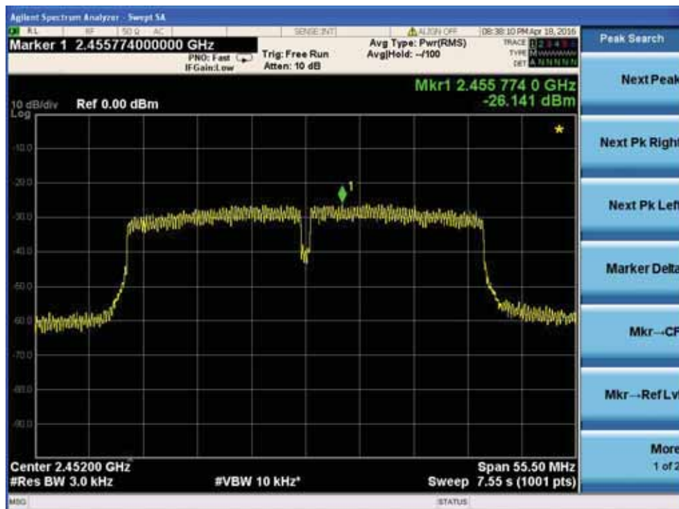
Power spectral density plot on channel 9
