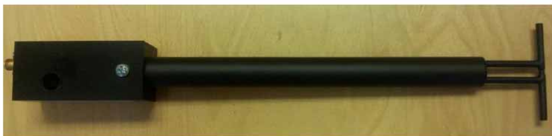
Figure 1 – MVG COMOSAR Validation Dipole
