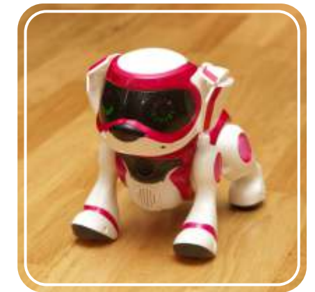
Vision sensors on a robotic dog
