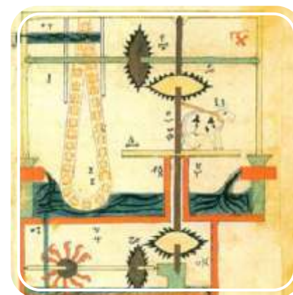
Al-Jazari's drawing of a hydropowered chain pump
