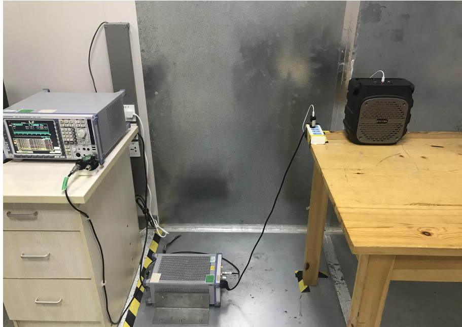
Radiated Spurious Emissions Test Frequency From Below 30MHz
