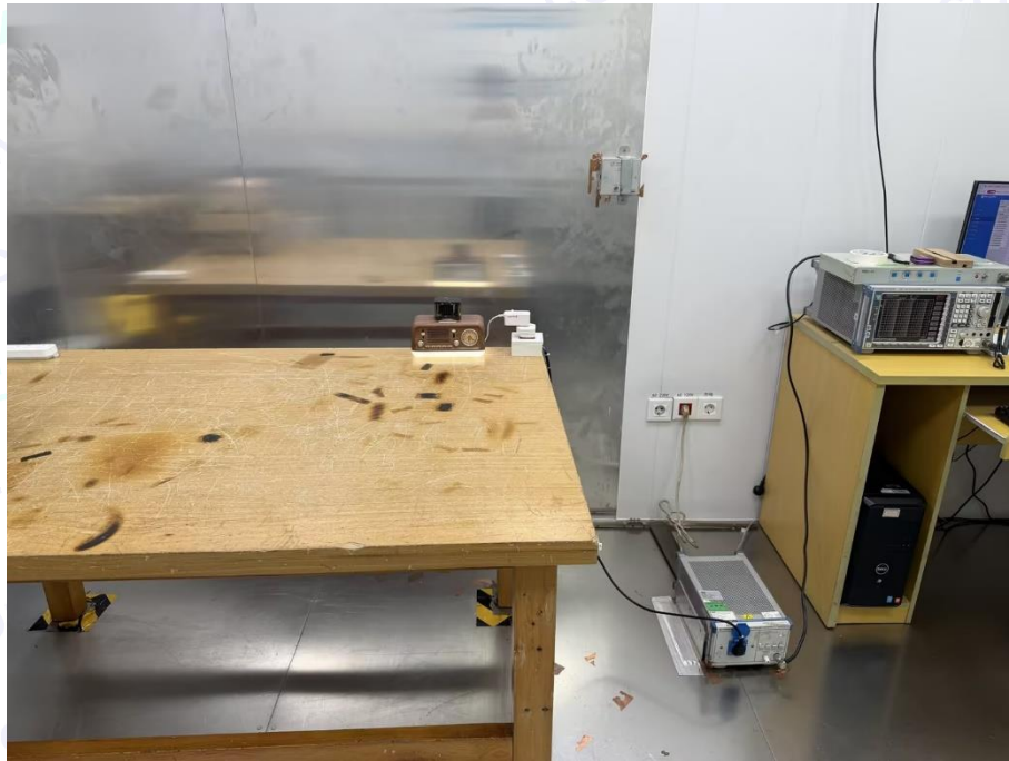
Photo of Setup for Conducted Emission(AC POWER)-WPT
