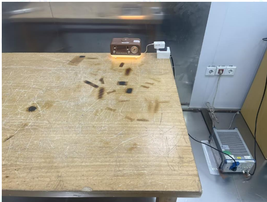
Photo of Setup for Radiated Emission (30MHz~1GHz)
