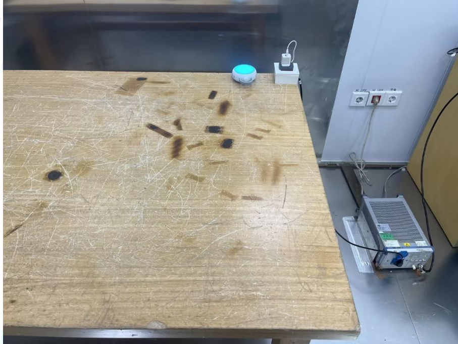
Photo of Setup for Radiated Emission (30MHz~1GHz)
