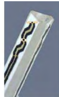
Figure 3.3 Probe Thick-Film Technique
