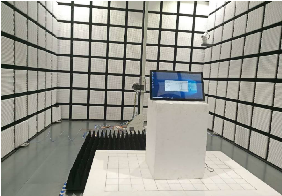
Fig. 3 Radiated emission setup photo(Above 1GHz)
