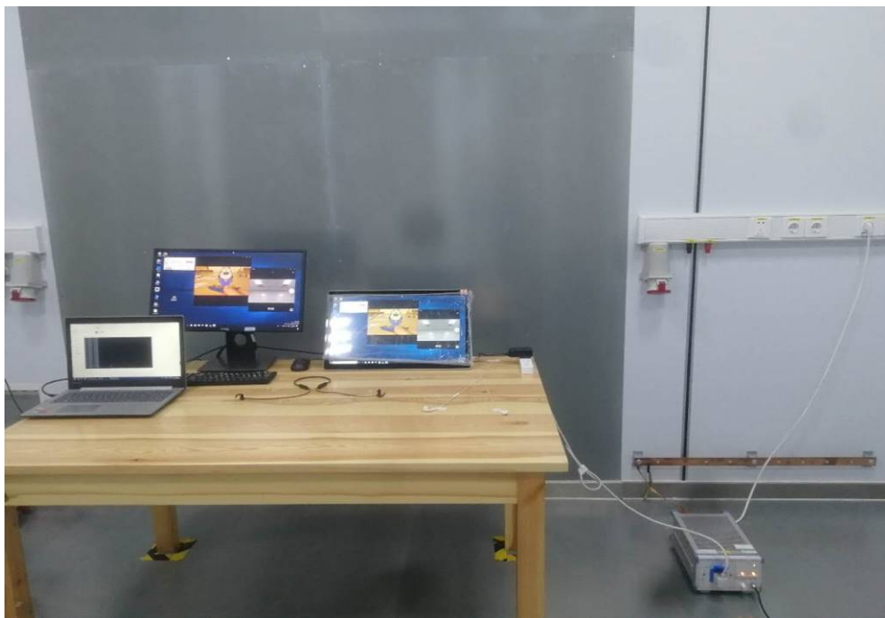
Fig. 4 Power line conducted emission setup photo
