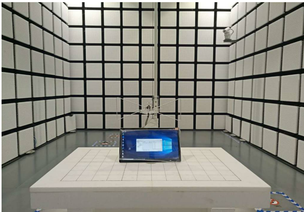
Fig. 2 Radiated emission setup photo(30MHz-1GHz)
