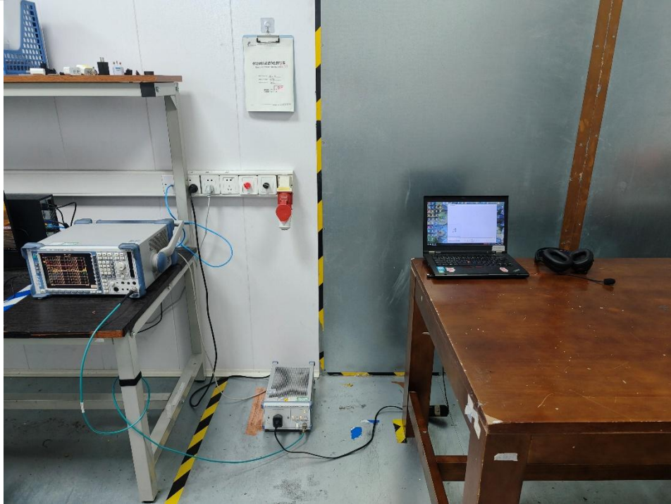
Conducted emissions at AC power line (150kHz-30MHz)
