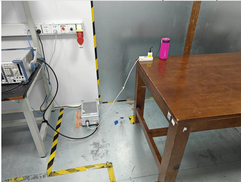
Conducted Emissions at Mains Terminals (150 kHz-30MHz)
