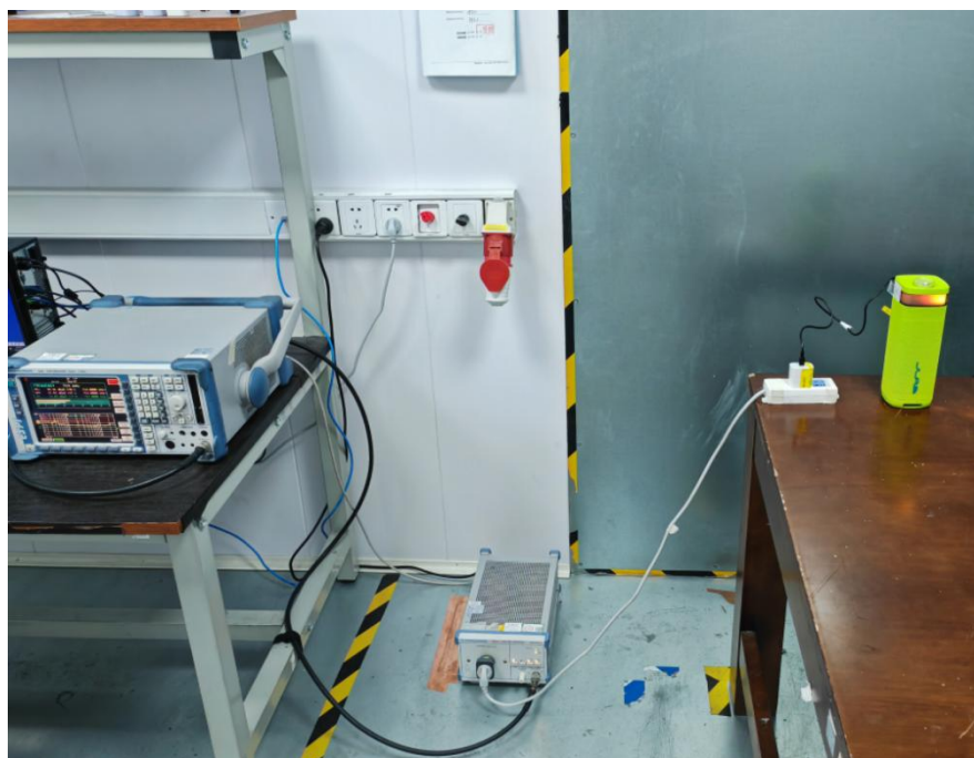
Conducted Emissions at Mains Terminals (150 kHz-30MHz)
