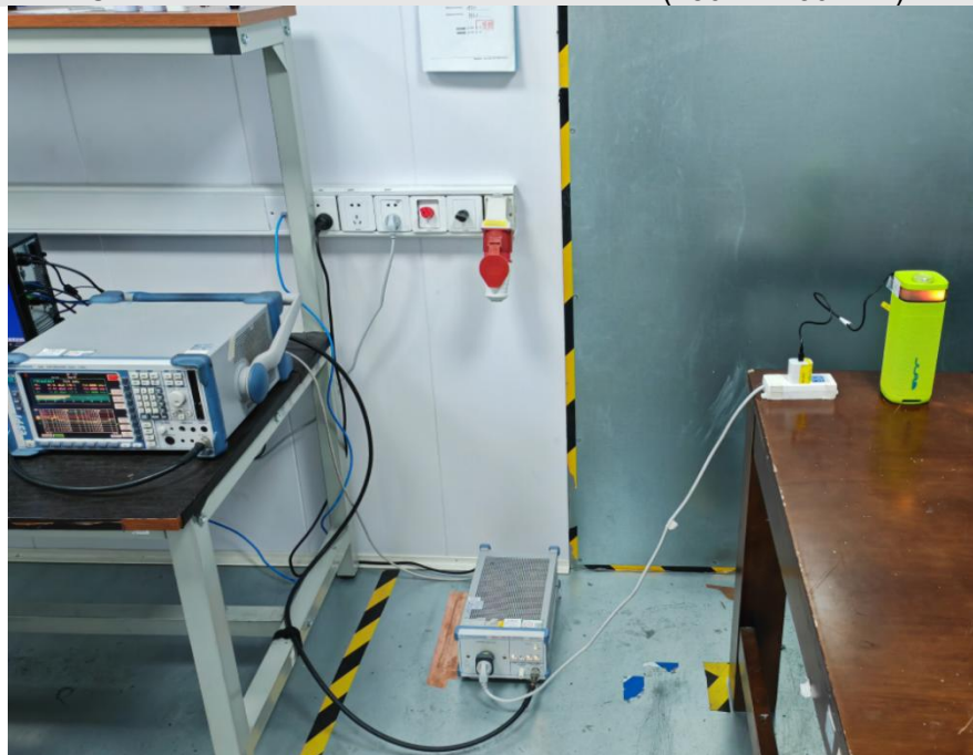
Conducted Emissions at Mains Terminals (150 kHz-30MHz)
