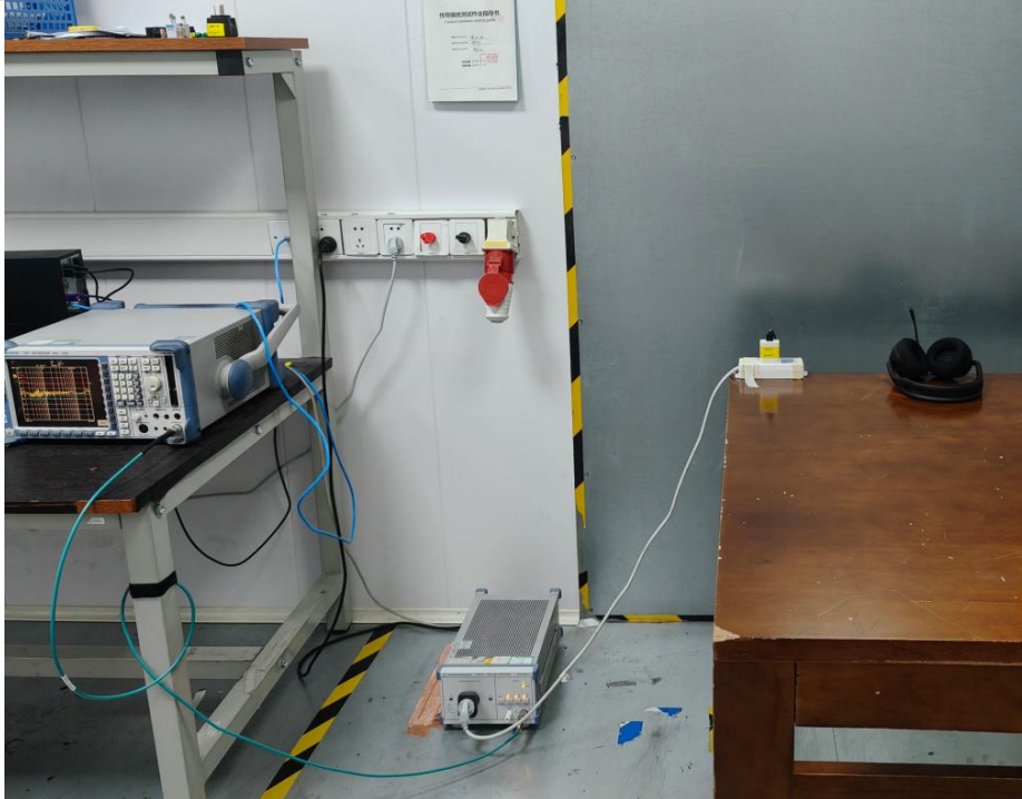
Conducted emissions at AC power line (150kHz-30MHz)
