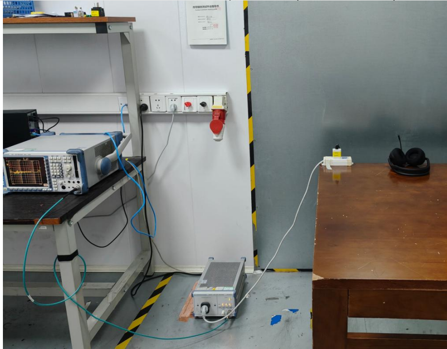
Conducted emissions at AC power line (150kHz-30MHz)
