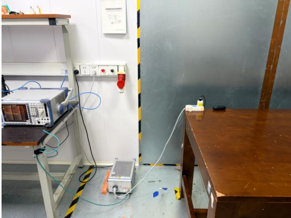
Conducted emissions at AC power line (150kHz-30MHz)
