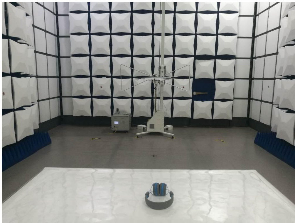
FCC RADIATED EMISSION TEST SETUP
