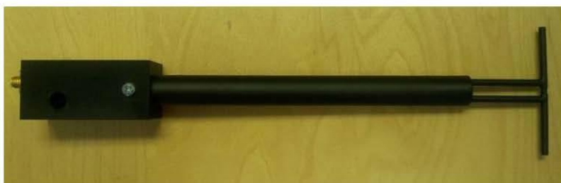
Figure 1 – MVG COMOSAR Validation Dipole
