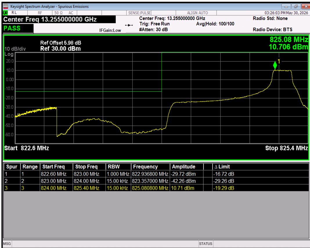
Band5 QPSK BW=1.4MHz Channel=20643 RB Size=1 Position=#0
