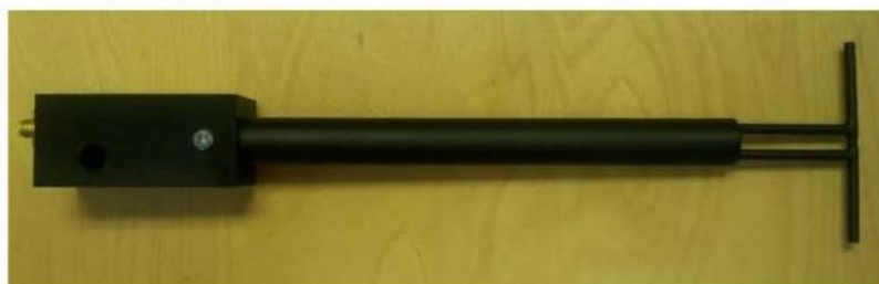
Figure 1 – MVG COMOSAR Validation Dipole
