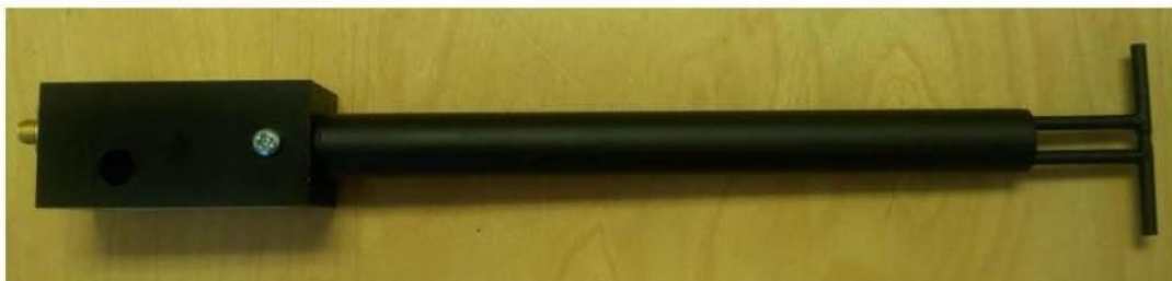
Figure 1 – MVG COMOSAR Validation Dipole
