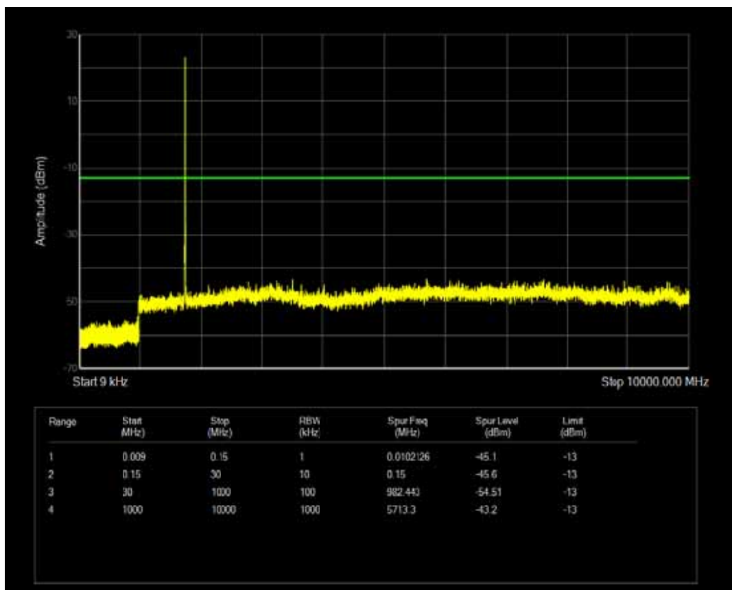
Band4 QAM16 BW=3MHz Channel=20385 RB Size=1 Position=#0
