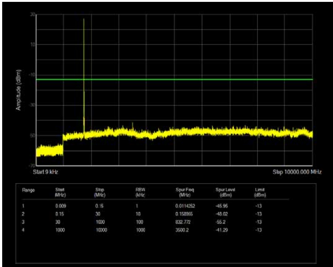
Band4 QPSK BW=5MHz Channel=20375 RB Size=25 Position=#0
