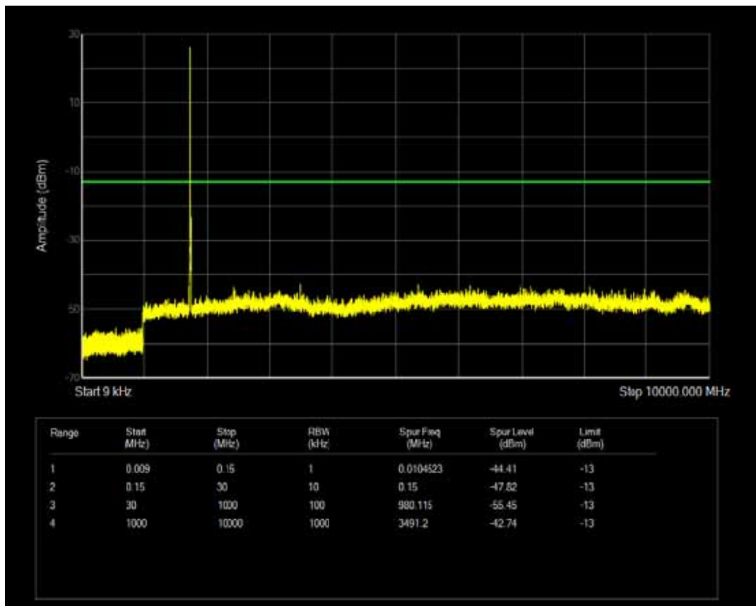
Band4 QPSK BW=15MHz Channel=20025 RB Size=1 Position=#0
