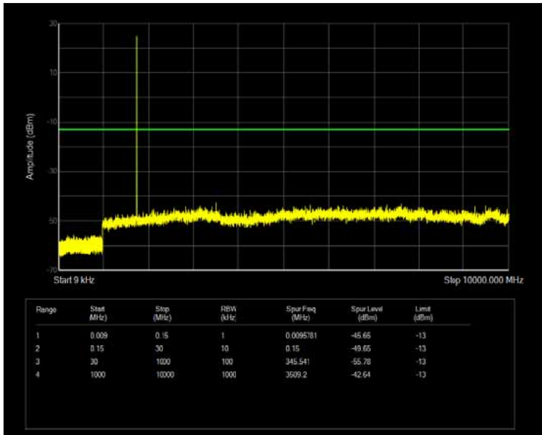
Band4 QPSK BW=3MHz Channel=19965 RB Size=15 Position=#0
