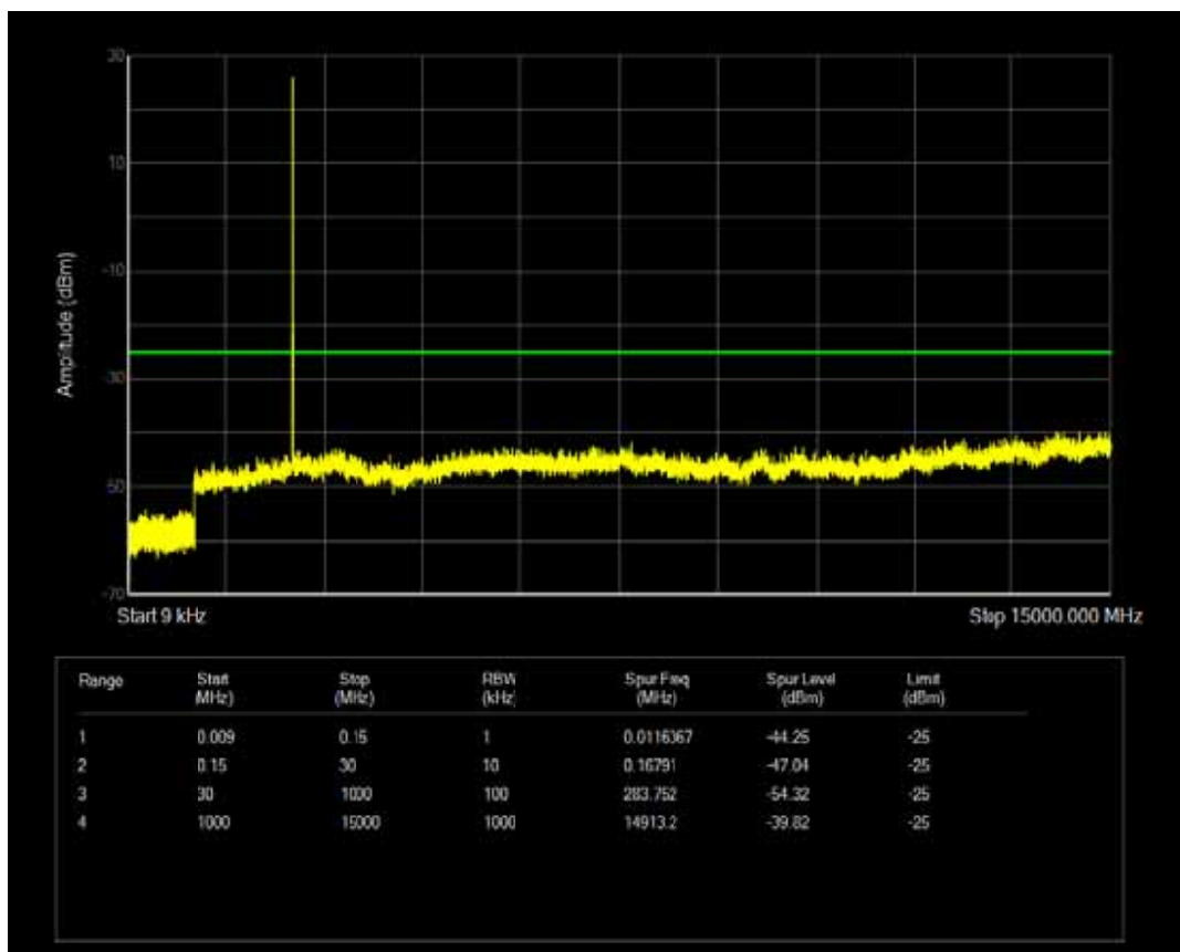
Band7 QAM16 BW=5MHz Channel=21100 RB Size=1 Position=#0
