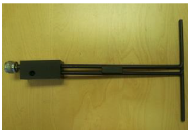
Figure 1 – MVG COMOSAR Validation Dipole
