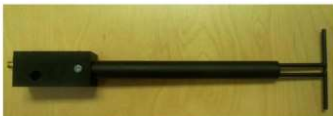
Figure 1 – MVG COMOSAR Validation Dipole
