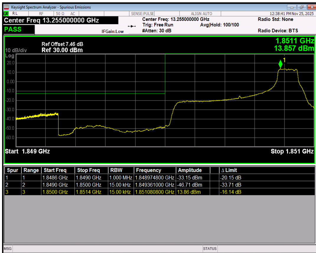
Band2 16QAM BW=1.4MHz Channel=18607 RB Size=6 Position=#0
