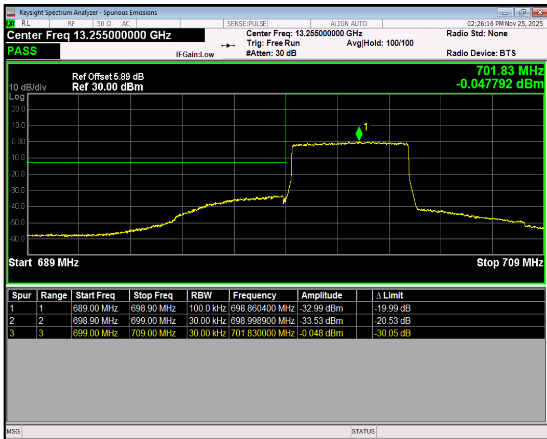
Band12 16QAM BW=5MHz Channel=23035 RB Size=1 Position=#0
