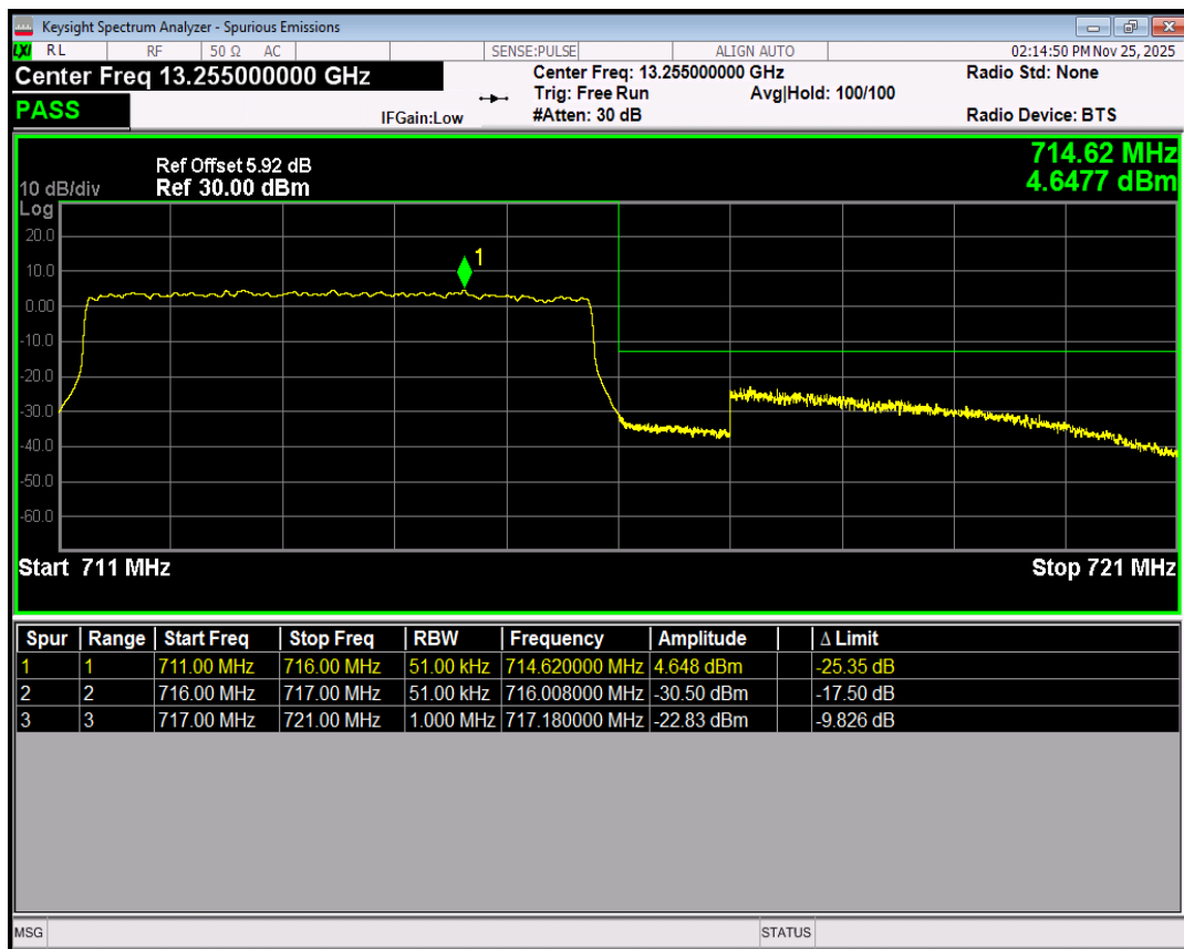
Band17 16QAM BW=5MHz Channel=23825 RB Size=1 Position=#0
