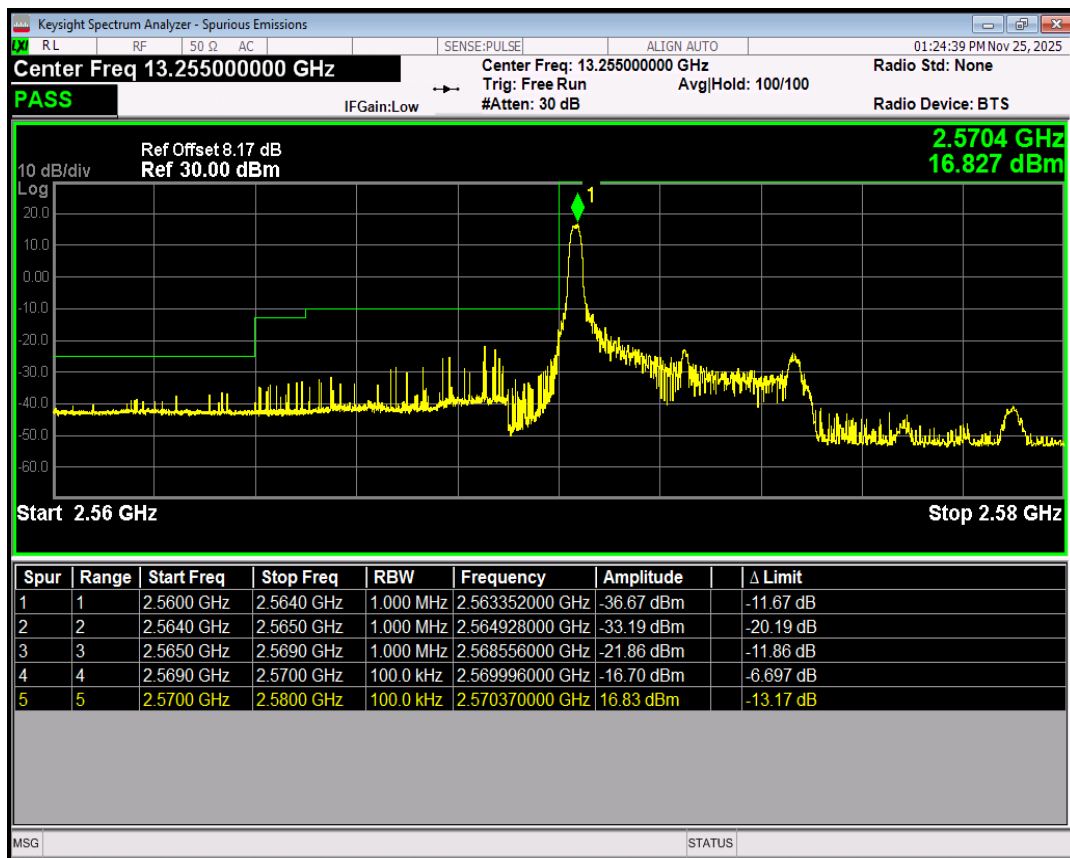
Band38 QPSK BW=5MHz Channel=37775 RB Size=1 Position=#Max
