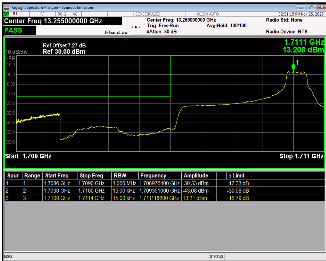
Band4 16QAM BW=1.4MHz Channel=19957 RB Size=6 Position=#0
