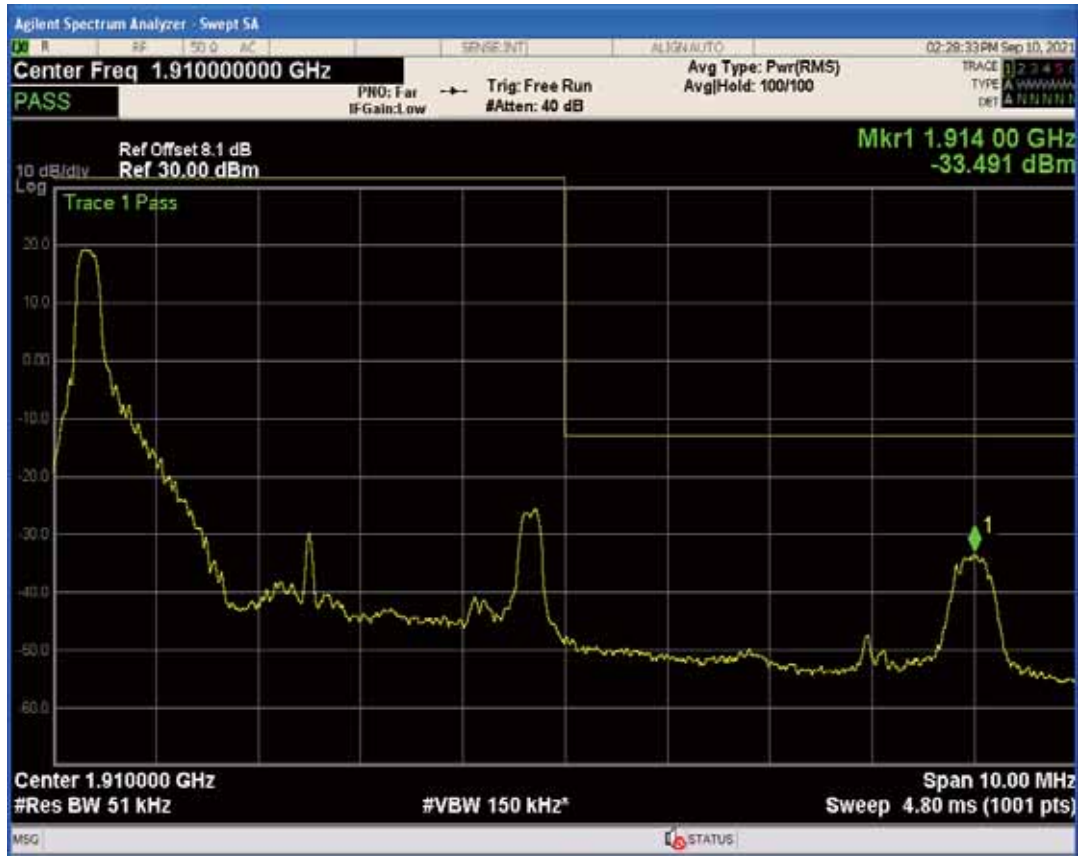
Band2 QPSK BW=5MHz Channel=19175 RB Size=25 Position=#0
