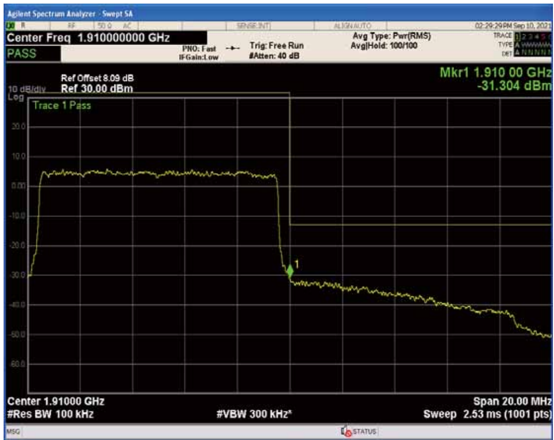
Band2 QPSK BW=10MHz Channel=19150 RB Size=1 Position=#Max
