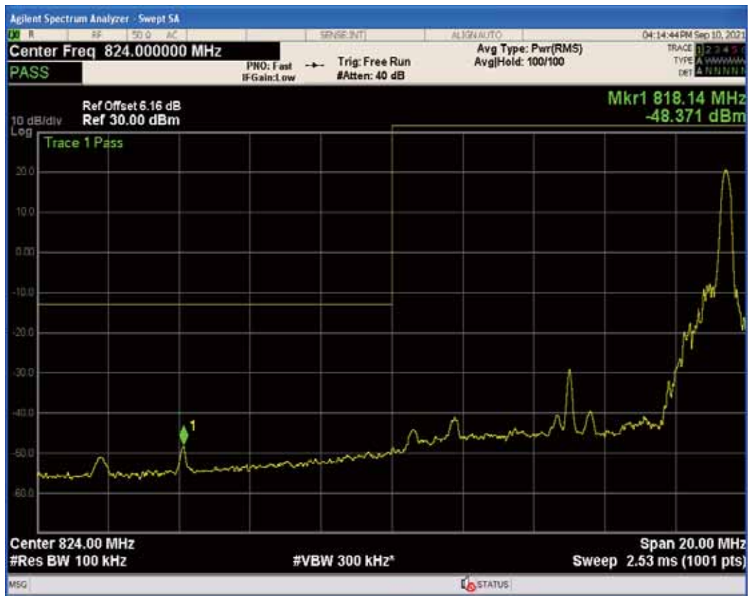
Band5 QAM16 BW=10MHz Channel=20450 RB Size=1 Position=#0
