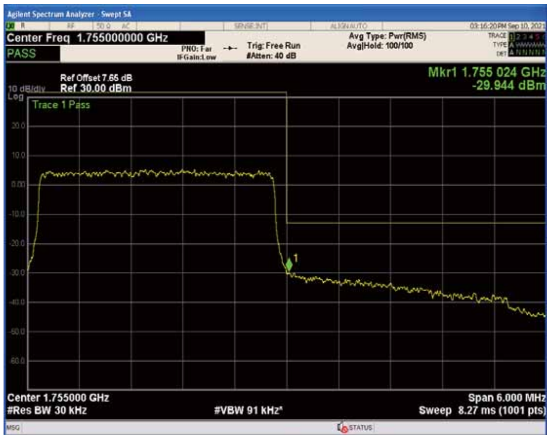
Band4 QAM16 BW=3MHz Channel=20385 RB Size=1 Position=#0
