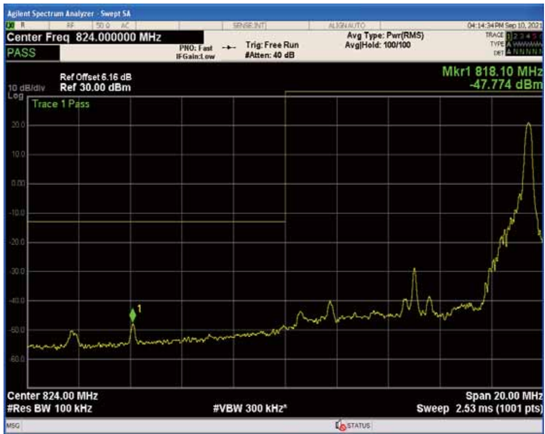
Band5 QPSK BW=10MHz Channel=20450 RB Size=50 Position=#0
