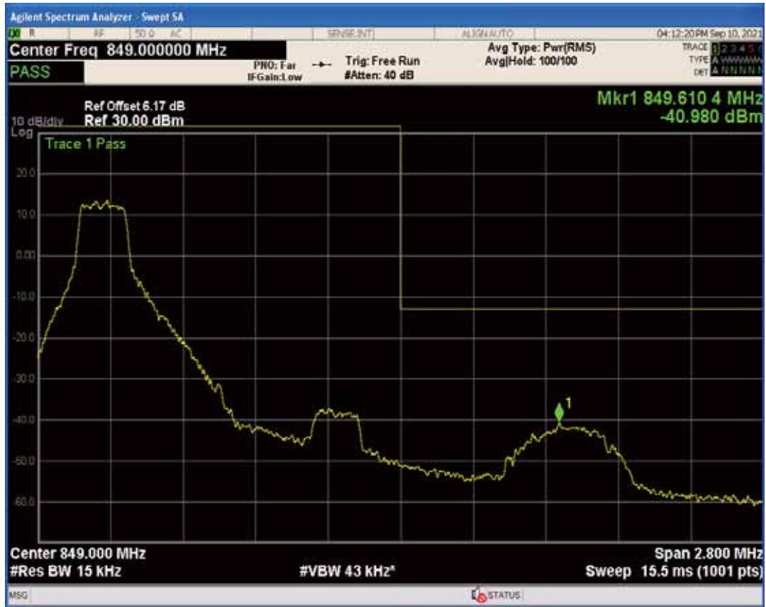
Band5 QAM16 BW=1.4MHz Channel=20643 RB Size=1 Position=#Max
