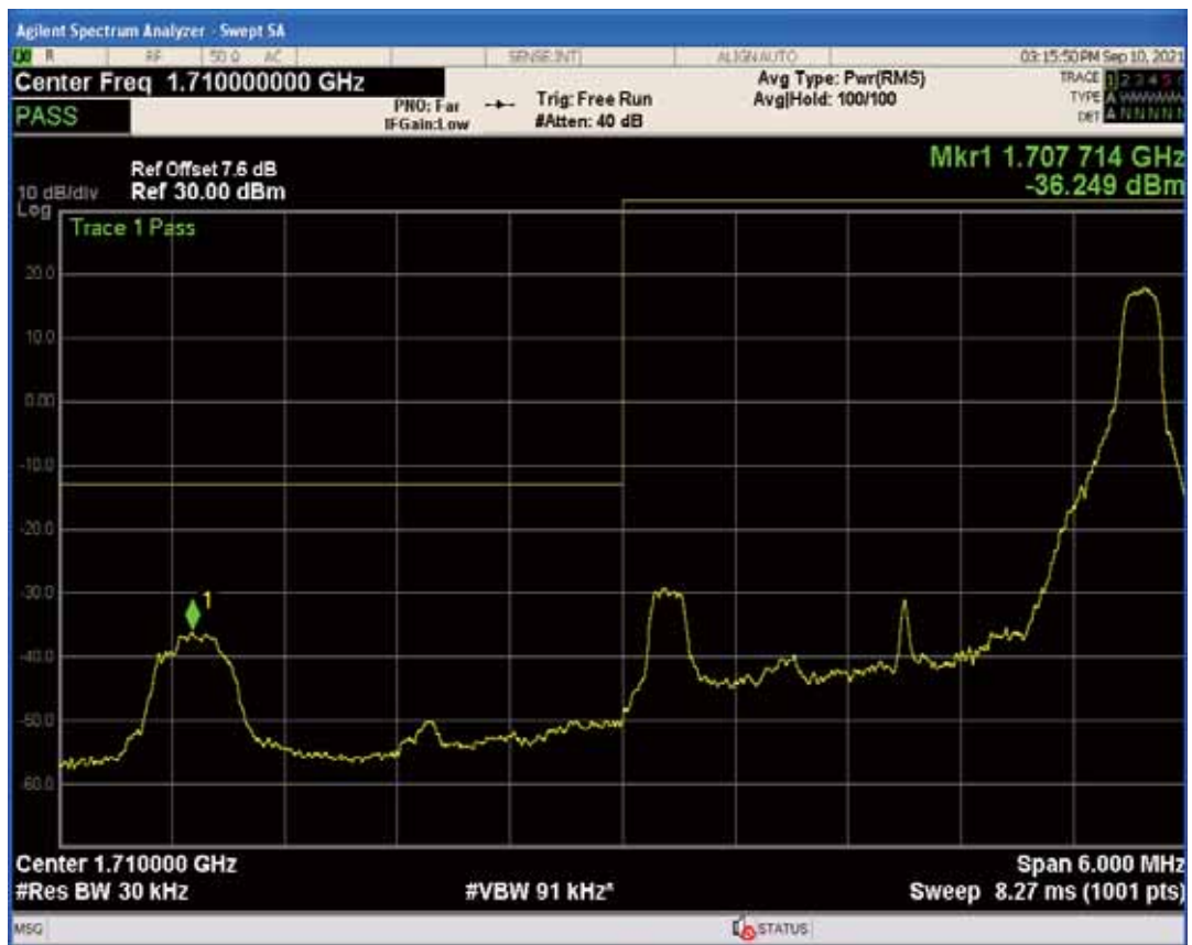
Band4 QAM16 BW=3MHz Channel=19965 RB Size=1 Position=#0
