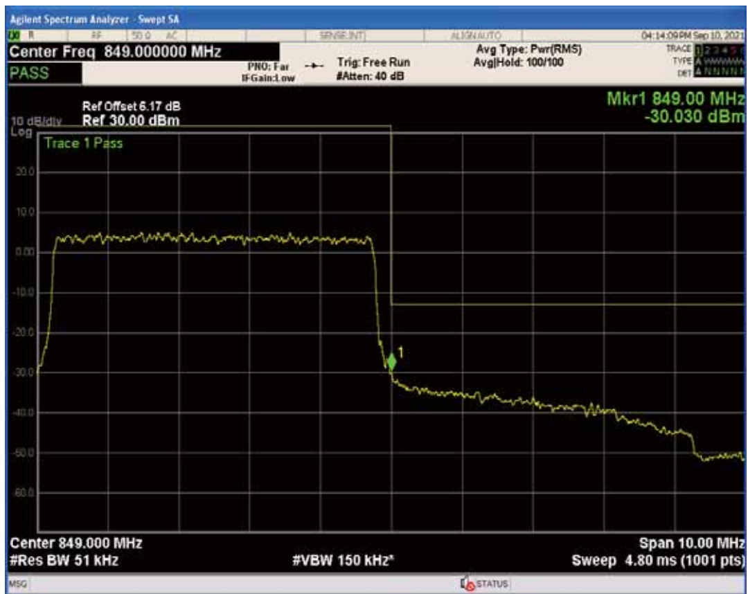
Band5 QAM16 BW=5MHz Channel=20625 RB Size=1 Position=#Max
