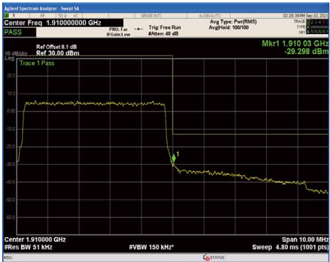
Band2 QAM16 BW=5MHz Channel=19175 RB Size=1 Position=#0
