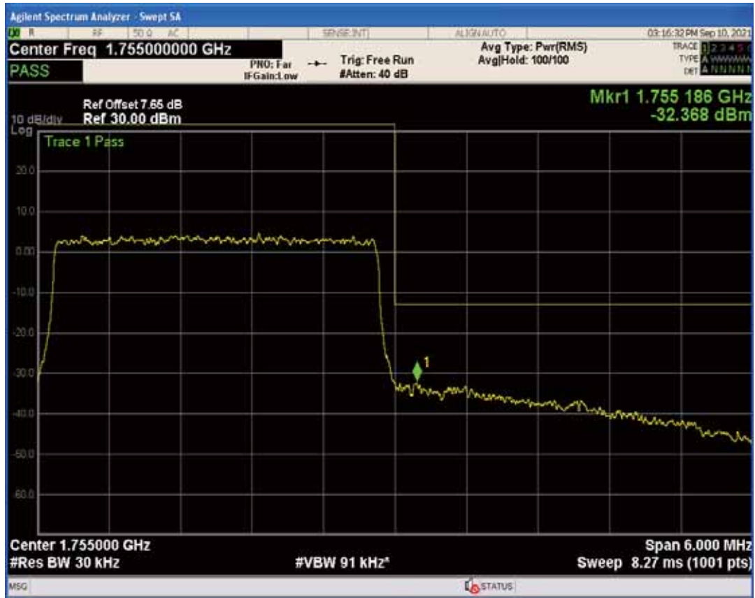
Band4 QPSK BW=5MHz Channel=19975 RB Size=1 Position=#Max
