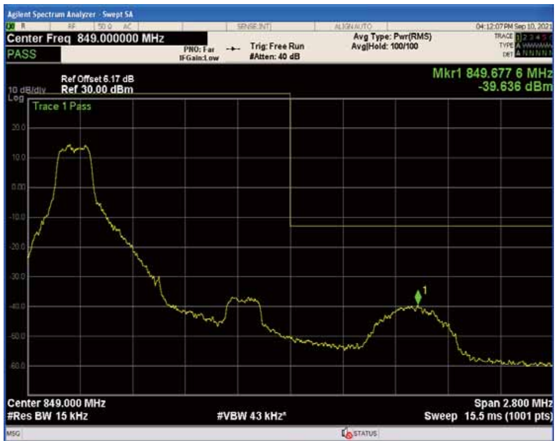
Band5 QPSK BW=1.4MHz Channel=20643 RB Size=1 Position=#Max
