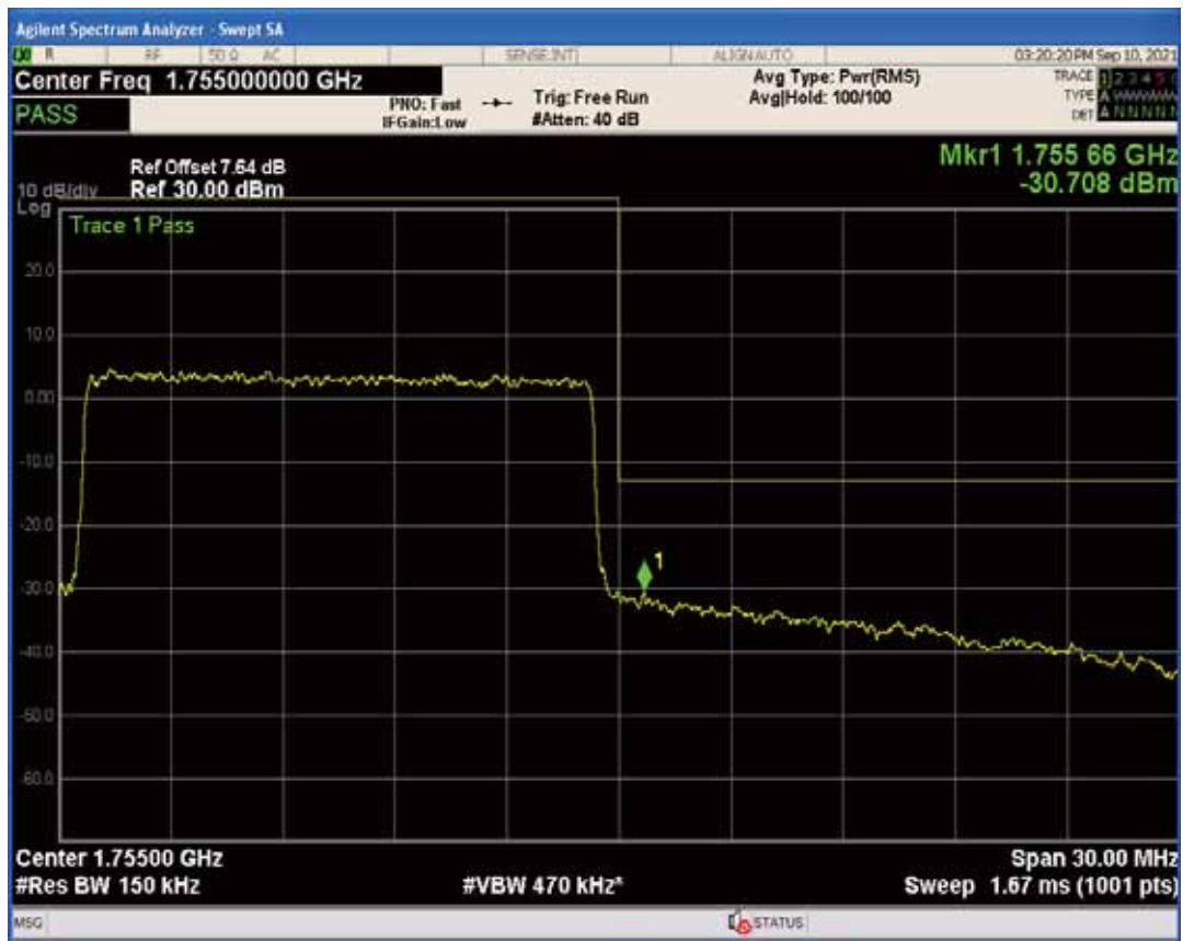
Band4 QPSK BW=20MHz Channel=20050 RB Size=1 Position=#Max
