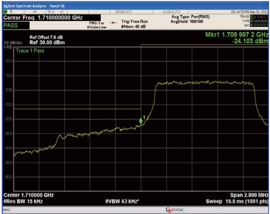
Band4 QAM16 BW=1.4MHz Channel=19957 RB Size=1 Position=#Max
