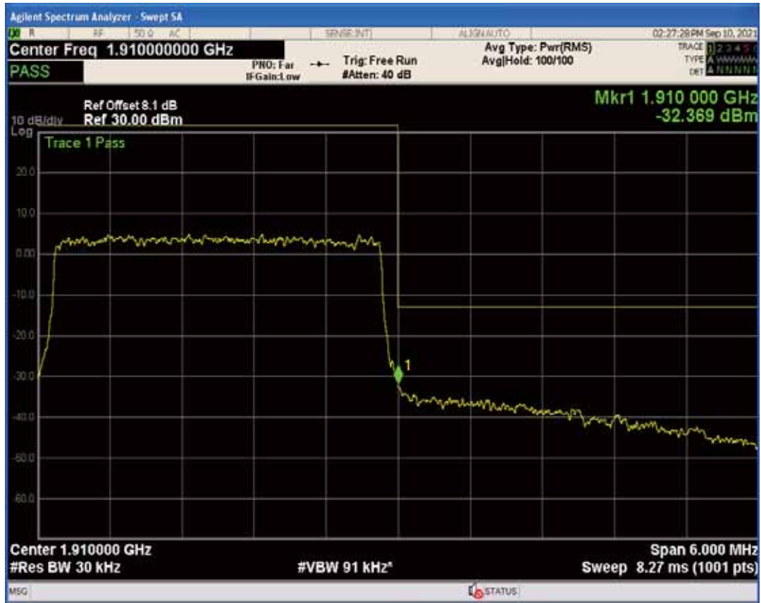
Band2 QPSK BW=5MHz Channel=18625 RB Size=1 Position=#0
