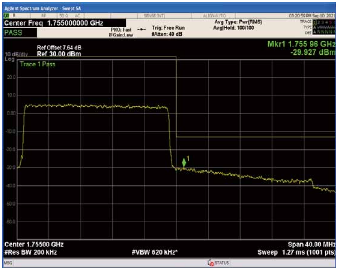
Band4 QAM16 BW=20MHz Channel=20300 RB Size=1 Position=#Max
