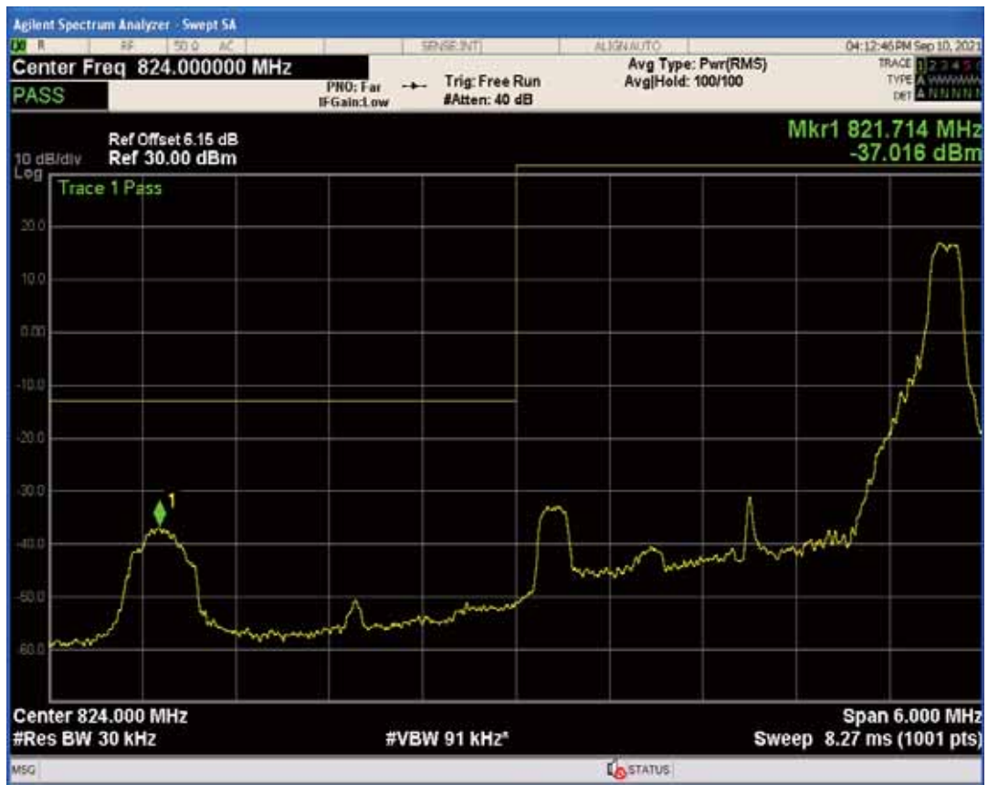
Band5 QPSK BW=3MHz Channel=20415 RB Size=15 Position=#0
