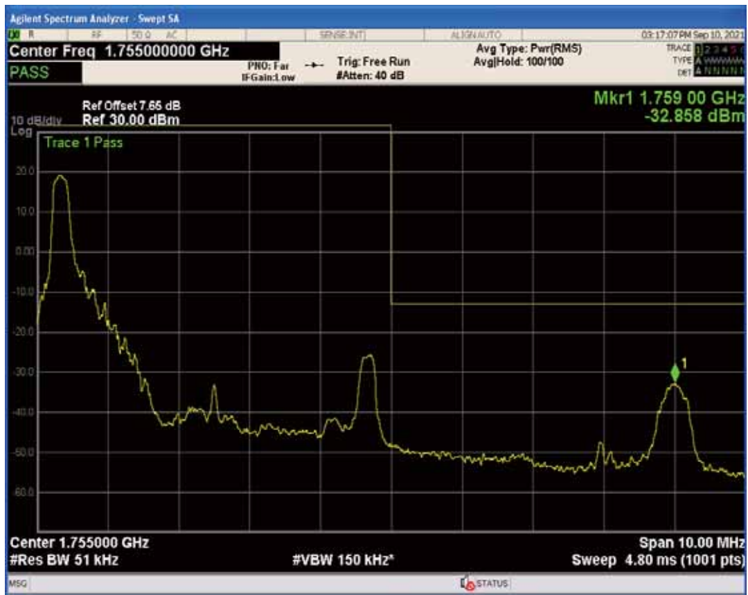
Band4 QAM16 BW=5MHz Channel=19975 RB Size=25 Position=#0
