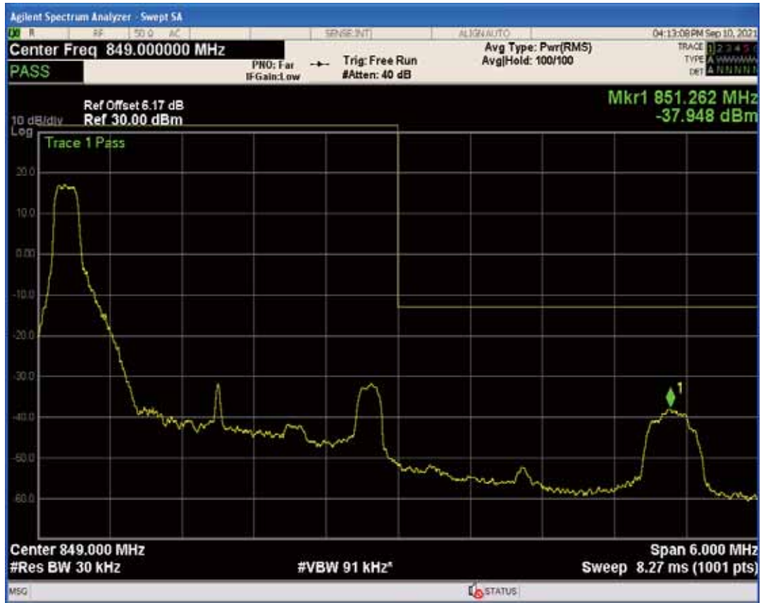
Band5 QAM16 BW=3MHz Channel=20415 RB Size=15 Position=#0
