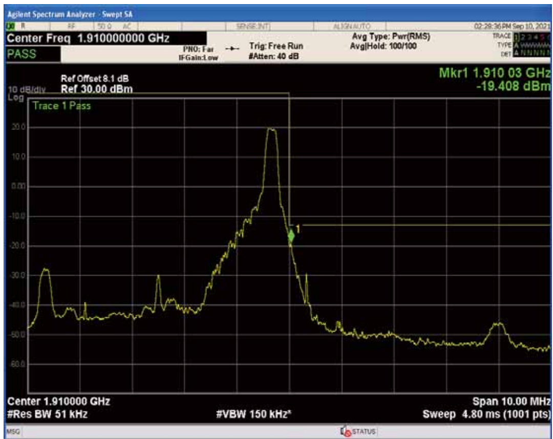
Band2 QPSK BW=5MHz Channel=19175 RB Size=1 Position=#0
