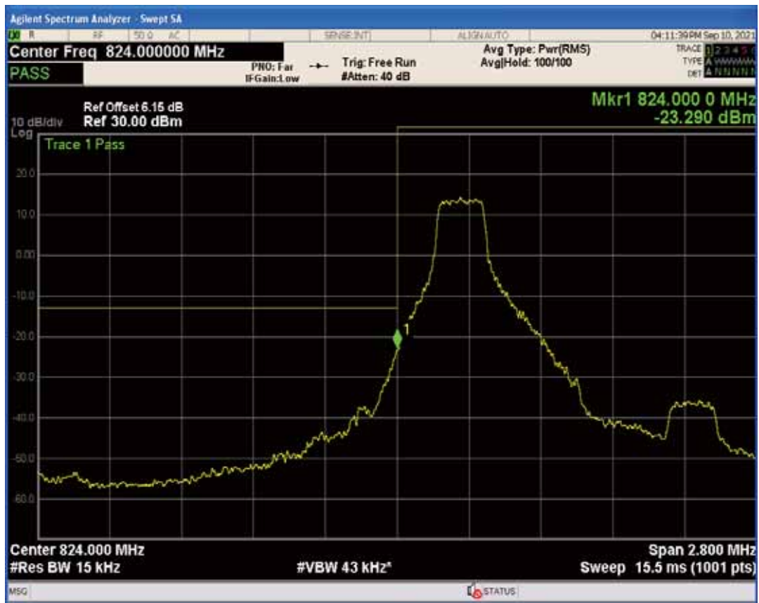
Band5 QPSK BW=1.4MHz Channel=20407 RB Size=6 Position=#0
