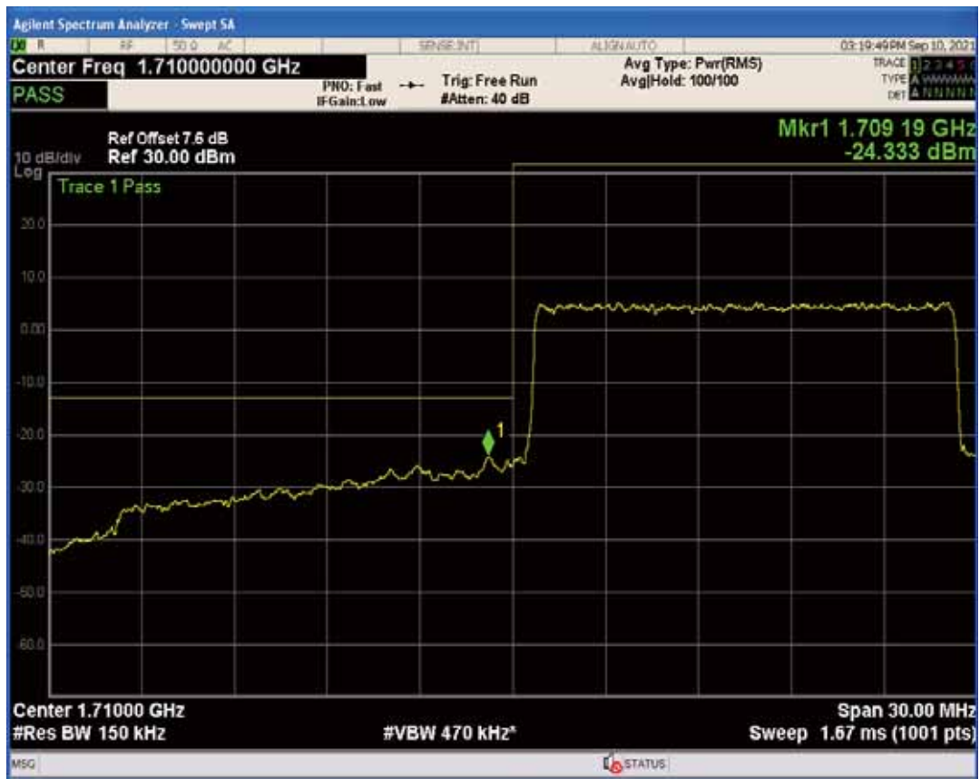
Band4 QPSK BW=15MHz Channel=20025 RB Size=1 Position=#Max
