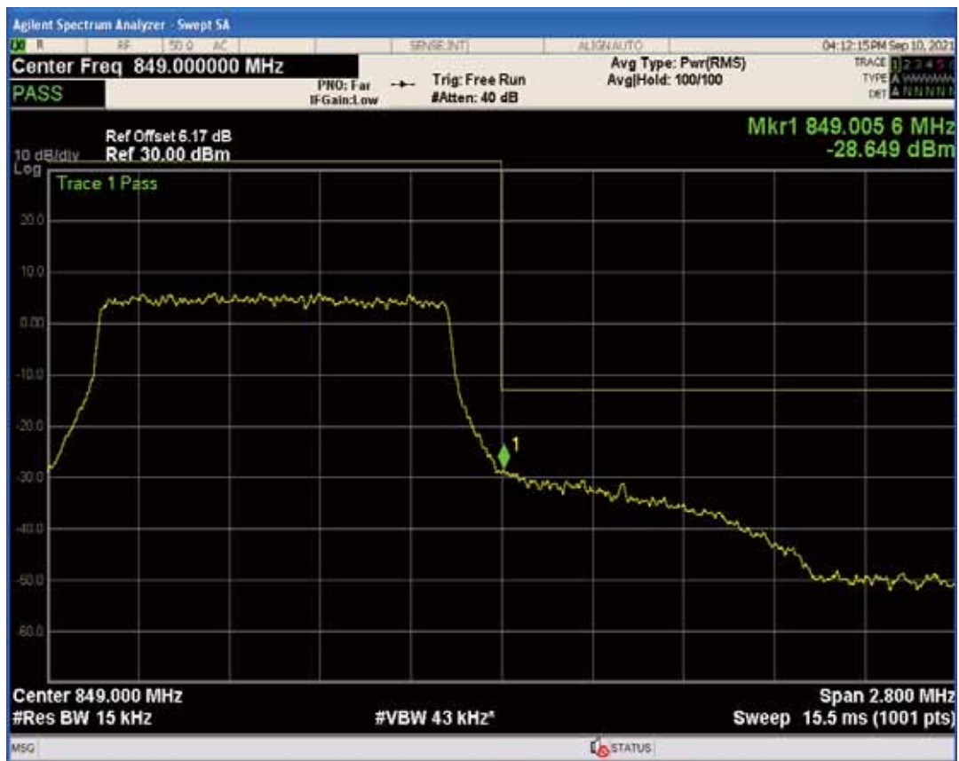
Band5 QAM16 BW=1.4MHz Channel=20643 RB Size=1 Position=#0
