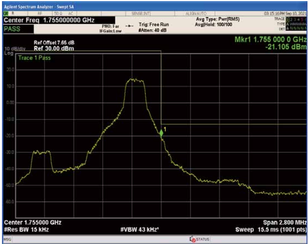
Band4 QAM16 BW=1.4MHz Channel=20393 RB Size=1 Position=#0
