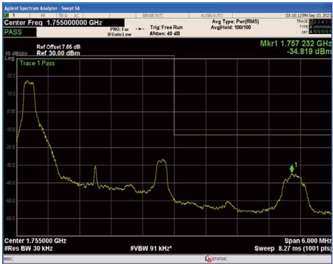
Band4 QPSK BW=3MHz Channel=20385 RB Size=15 Position=#0
