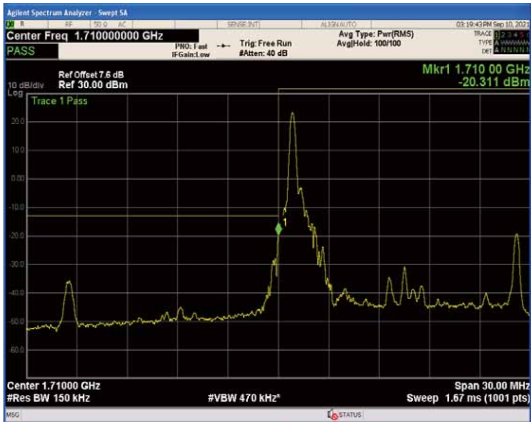
Band4 QPSK BW=15MHz Channel=20025 RB Size=75 Position=#0
