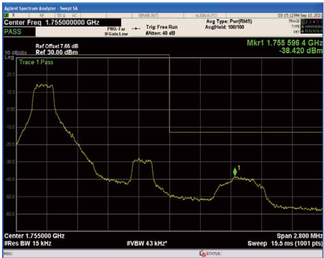
Band4 QPSK BW=1.4MHz Channel=20393 RB Size=1 Position=#Max
