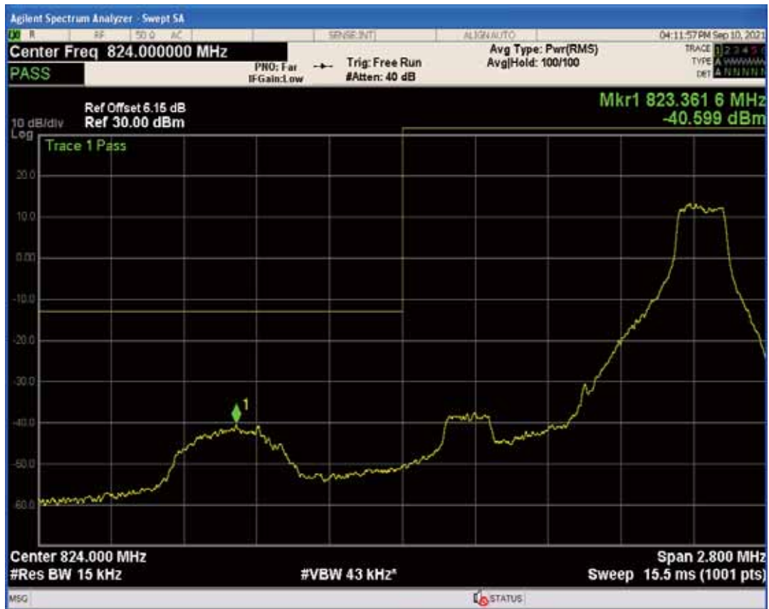
Band5 QAM16 BW=1.4MHz Channel=20407 RB Size=6 Position=#0
