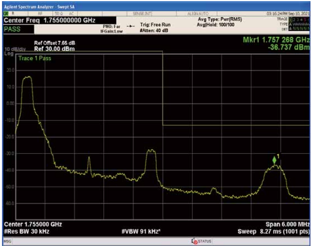
Band4 QAM16 BW=3MHz Channel=20385 RB Size=1 Position=#Max
