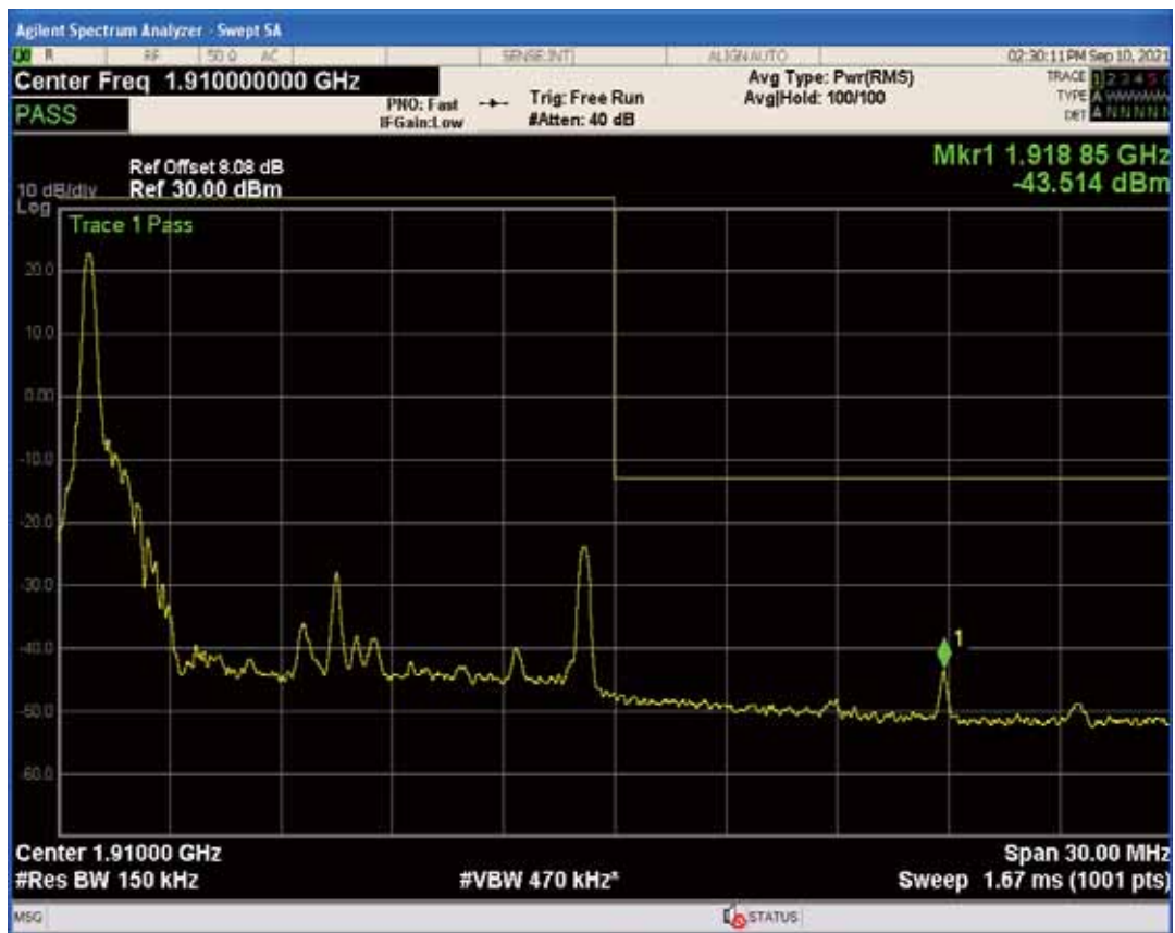
Band2 QPSK BW=15MHz Channel=19125 RB Size=1 Position=#Max
