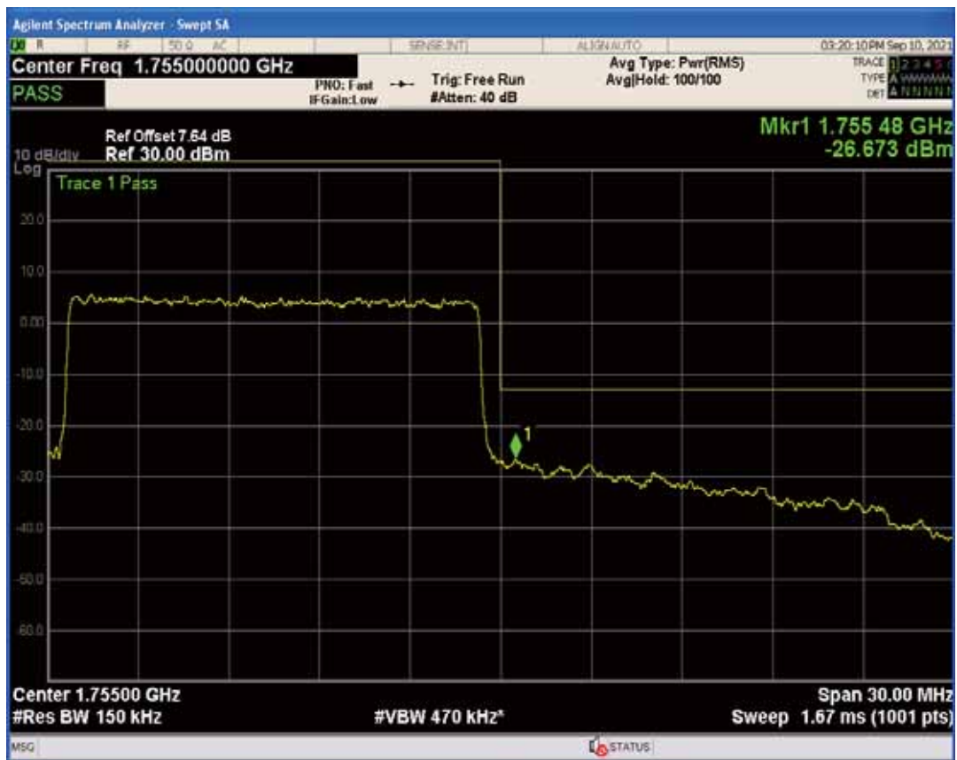
Band4 QAM16 BW=15MHz Channel=20325 RB Size=1 Position=#Max
