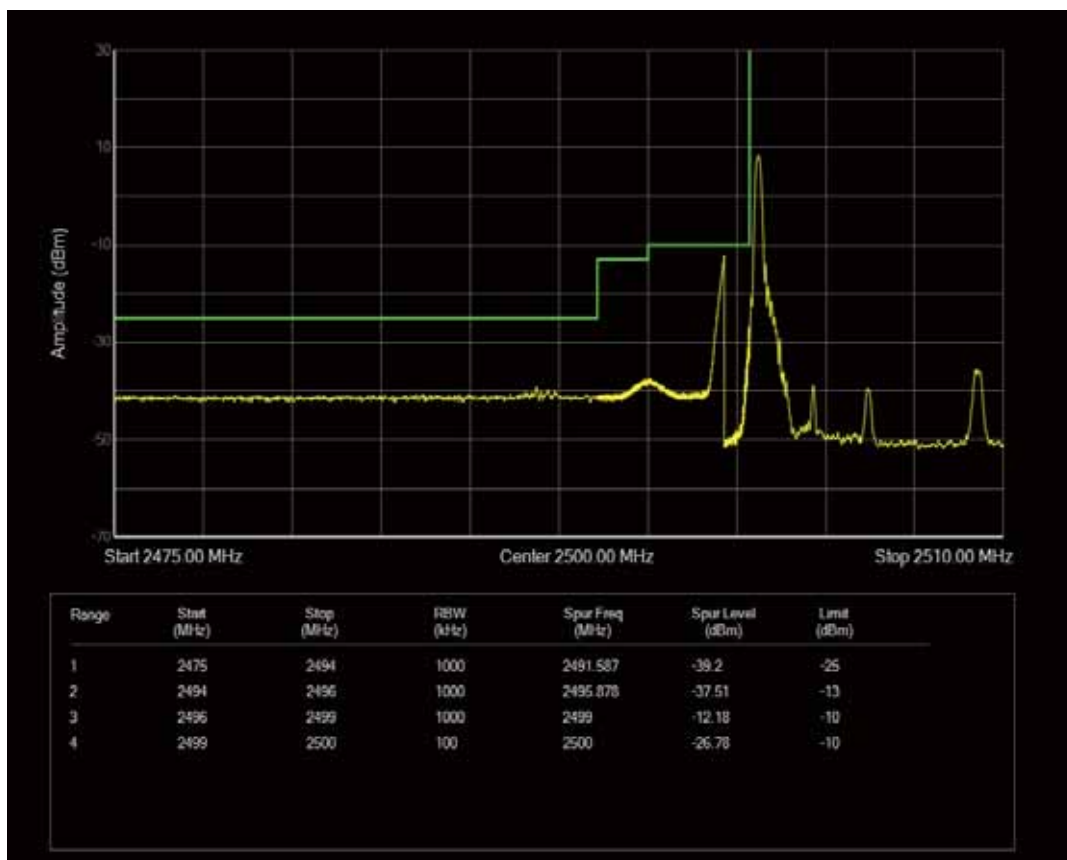
Band7 QPSK BW=5MHz Channel=20775 RB Size=25 Position=#0
