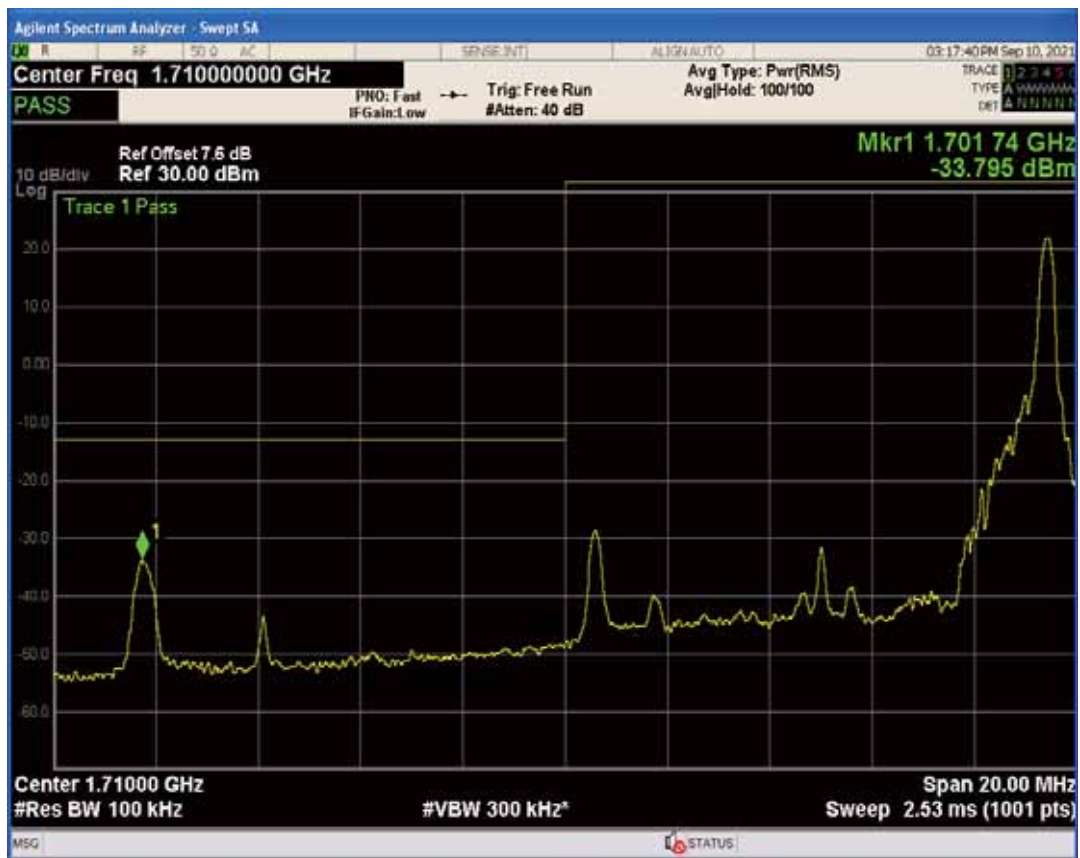
Band4 QAM16 BW=10MHz Channel=20000 RB Size=1 Position=#0
