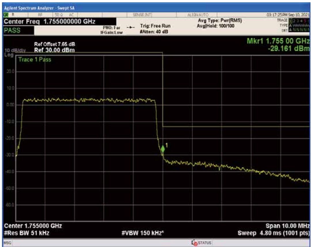
Band4 QPSK BW=10MHz Channel=20000 RB Size=50 Position=#0
