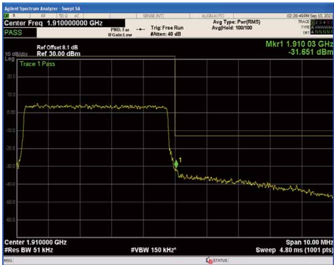
Band2 QPSK BW=10MHz Channel=18650 RB Size=1 Position=#Max
