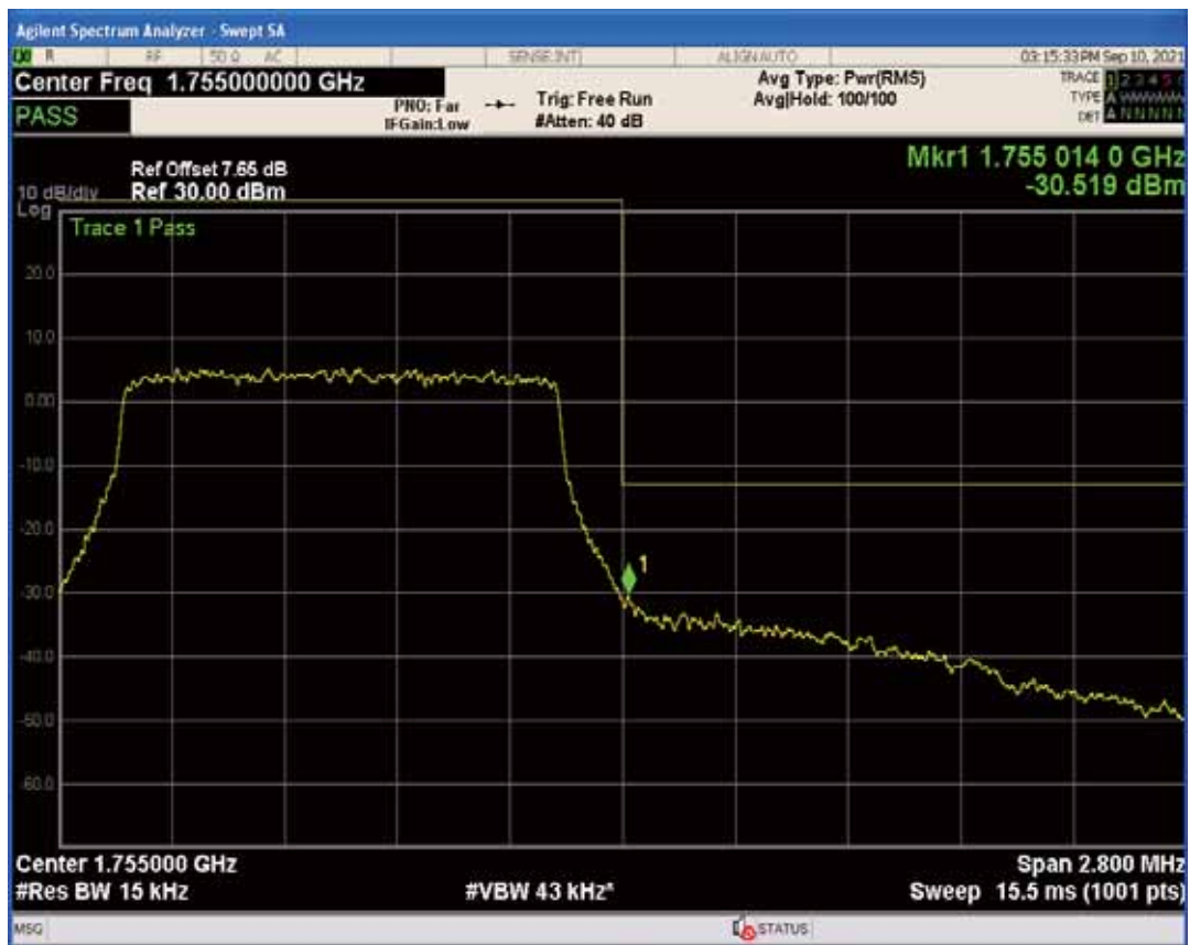
Band4 QAM16 BW=1.4MHz Channel=20393 RB Size=1 Position=#Max
