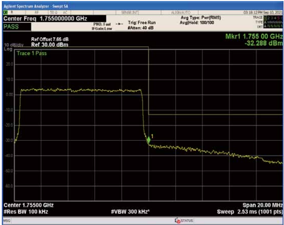
Band4 QPSK BW=15MHz Channel=20025 RB Size=1 Position=#0
