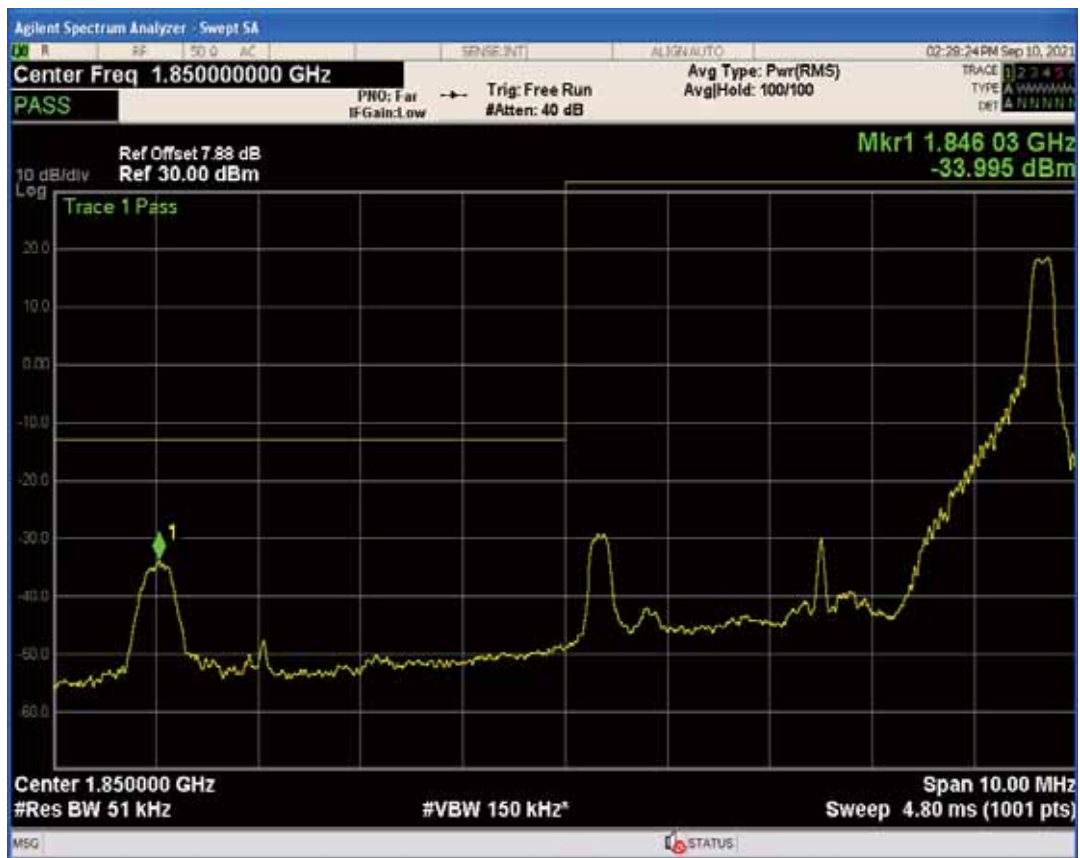
Band2 QAM16 BW=5MHz Channel=18625 RB Size=25 Position=#0
