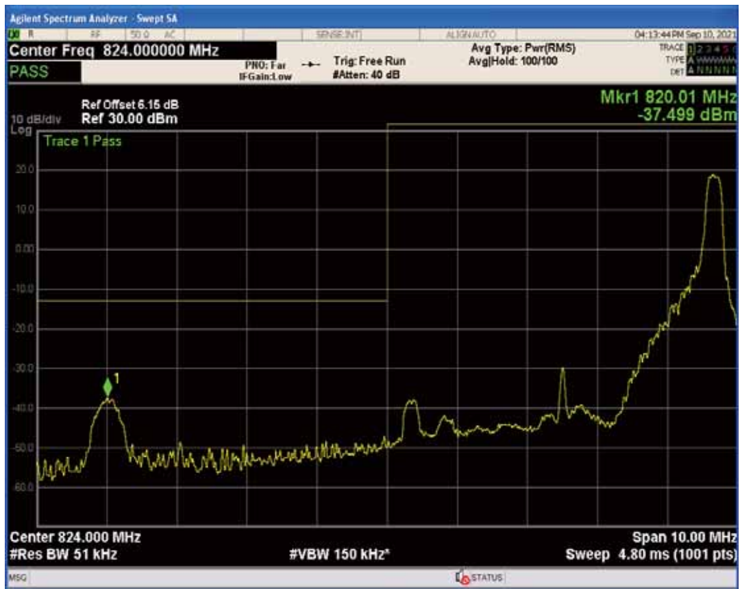
Band5 QAM16 BW=5MHz Channel=20425 RB Size=1 Position=#0
