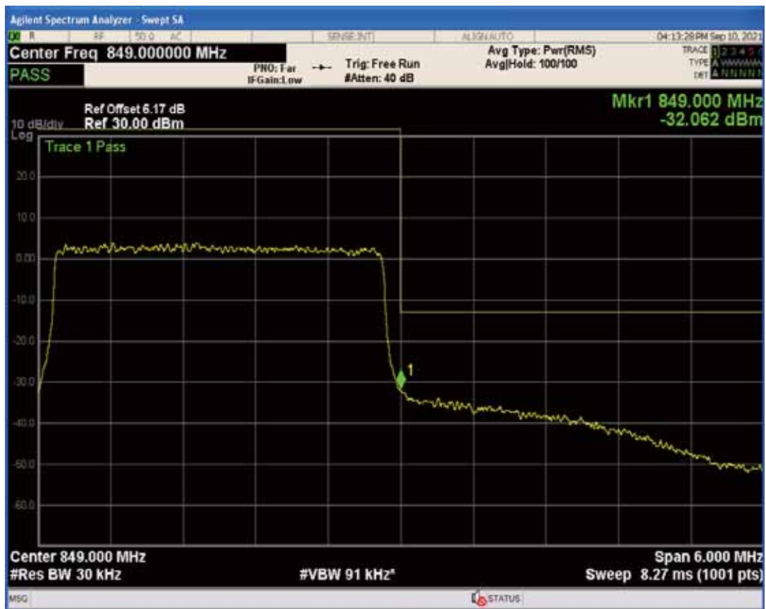
Band5 QPSK BW=5MHz Channel=20425 RB Size=1 Position=#Max
