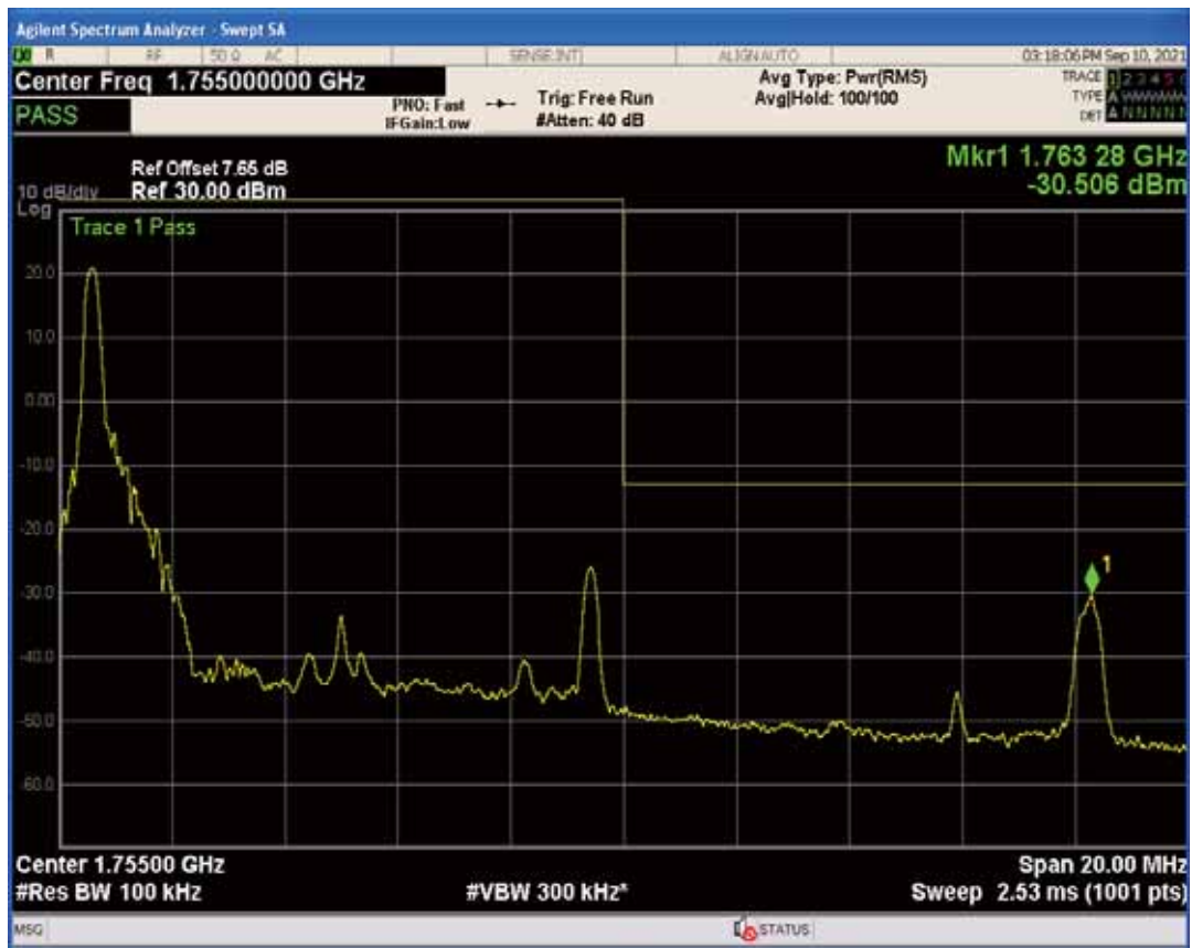
Band4 QAM16 BW=10MHz Channel=20350 RB Size=1 Position=#Max
