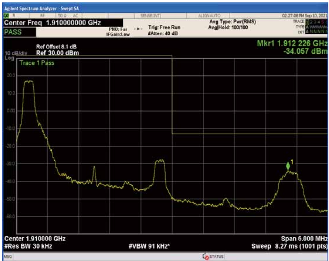
Band2 QPSK BW=3MHz Channel=19185 RB Size=1 Position=#Max
