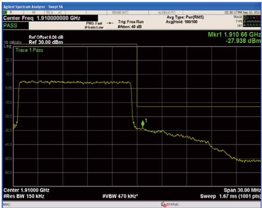
Band2 QAM16 BW=15MHz Channel=19125 RB Size=1 Position=#0
