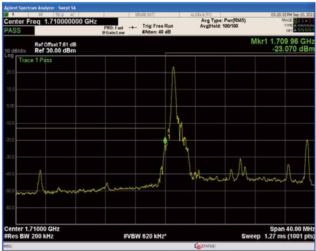
Band4 QPSK BW=20MHz Channel=20050 RB Size=100 Position=#0
