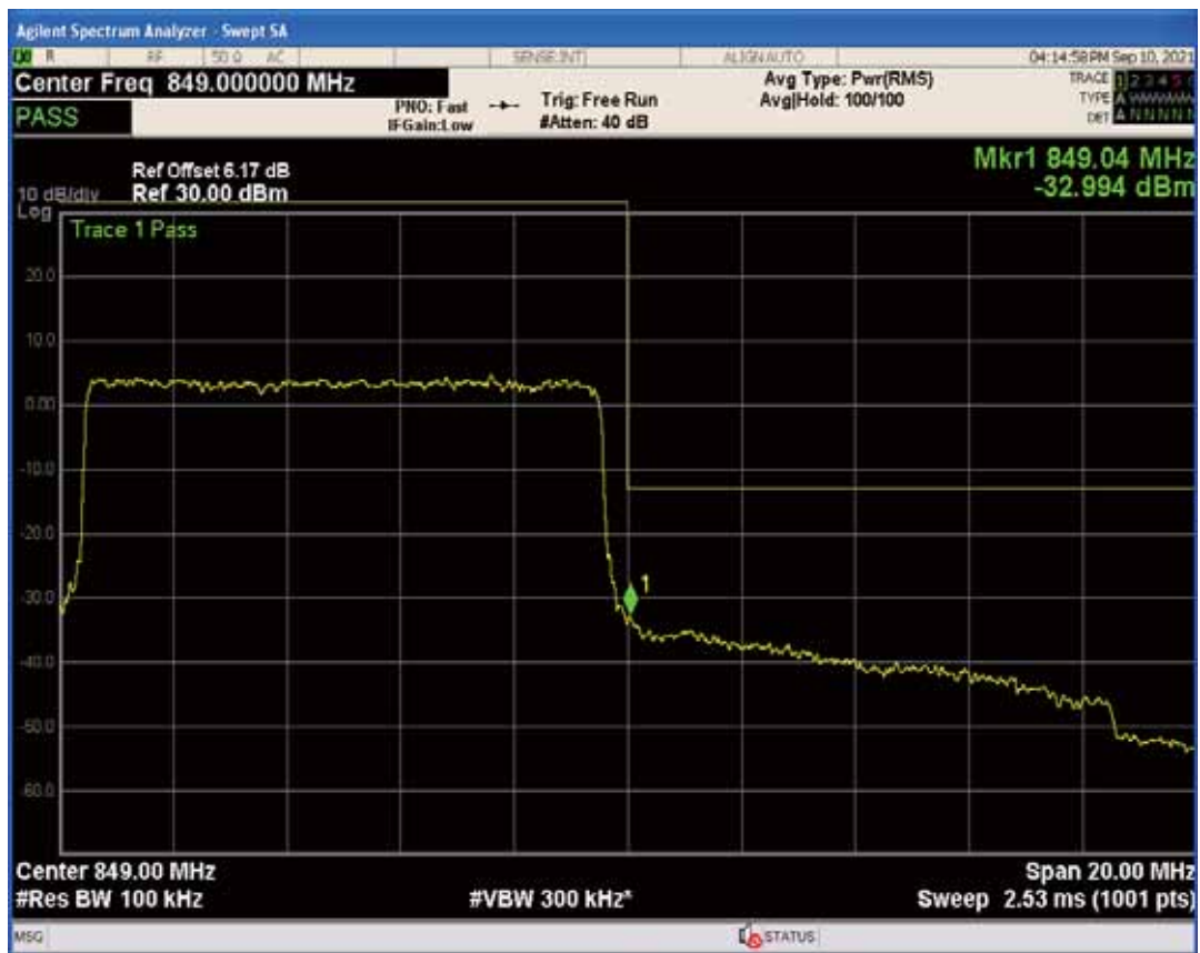
Band5 QAM16 BW=10MHz Channel=20600 RB Size=1 Position=#0
