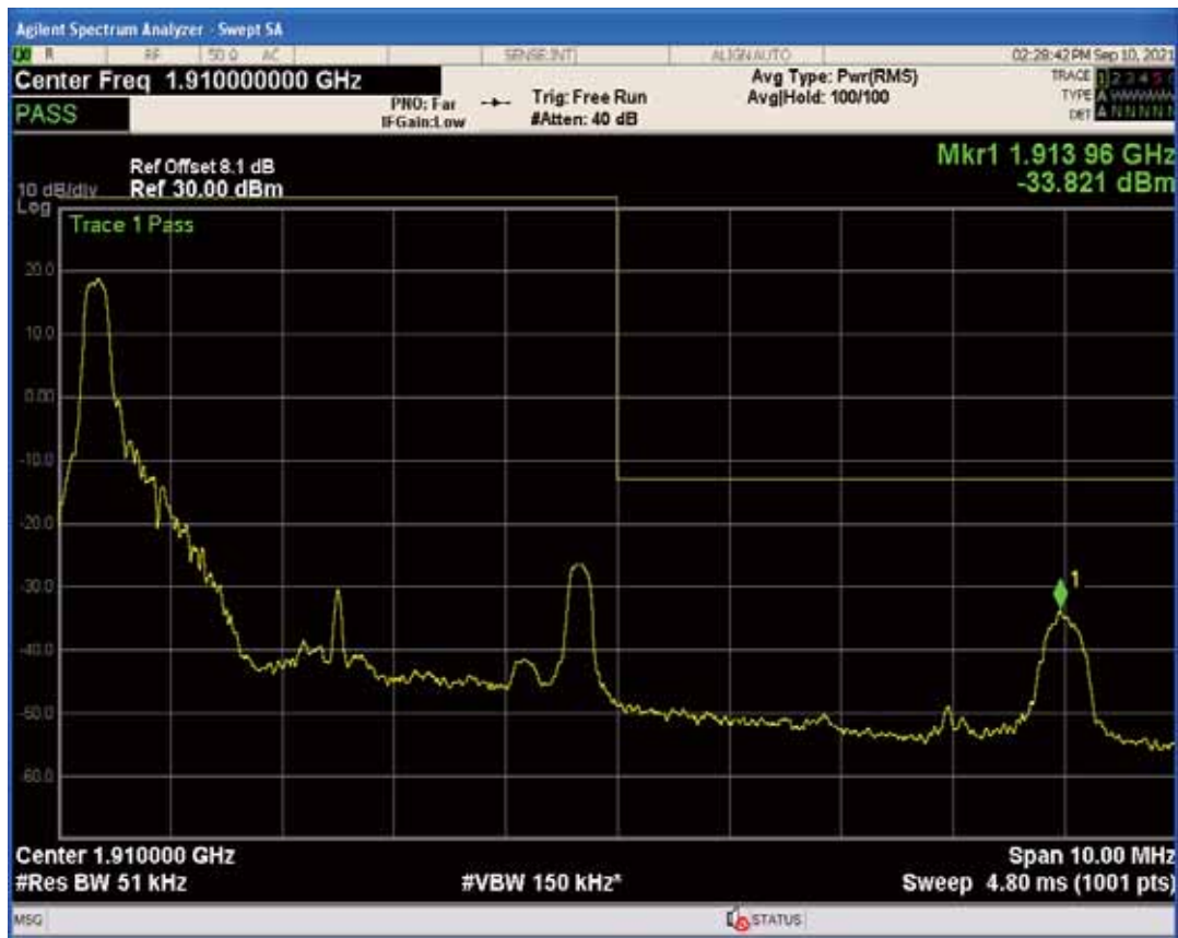
Band2 QAM16 BW=5MHz Channel=19175 RB Size=1 Position=#Max
