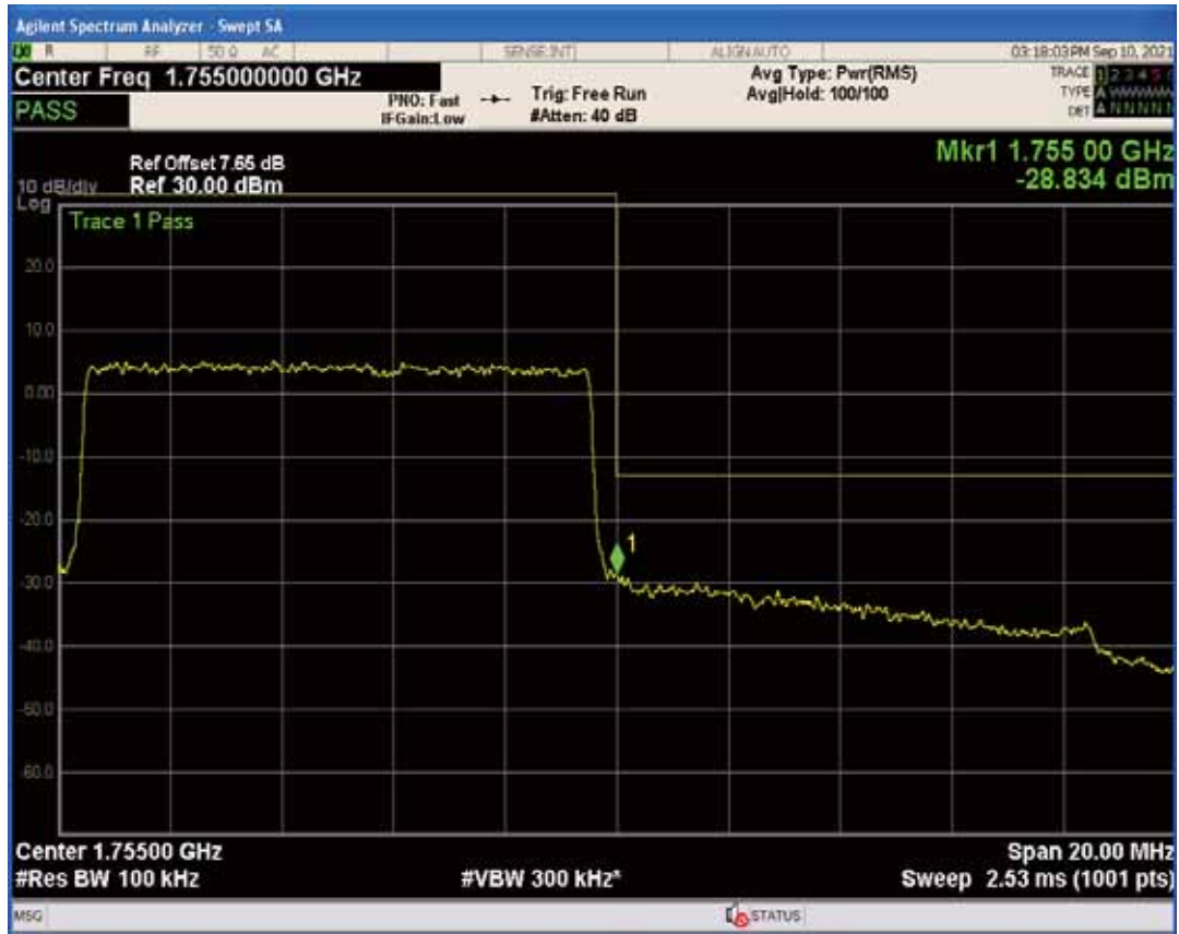
Band4 QPSK BW=10MHz Channel=20350 RB Size=1 Position=#Max
