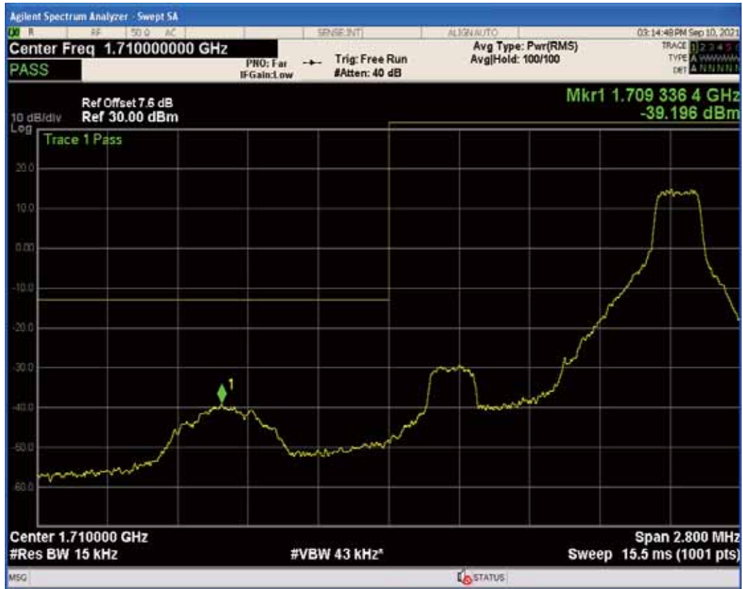
Band4 QAM16 BW=1.4MHz Channel=19957 RB Size=1 Position=#0
