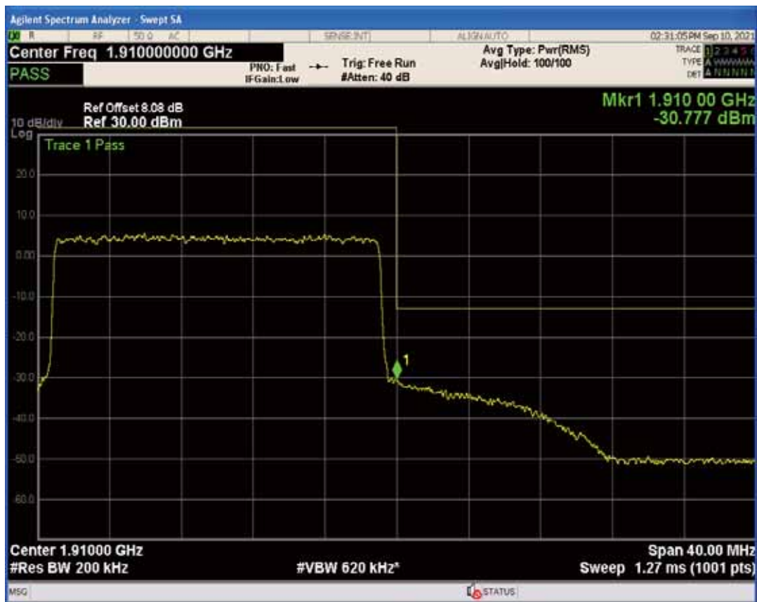
Band2 QAM16 BW=20MHz Channel=19100 RB Size=1 Position=#0
