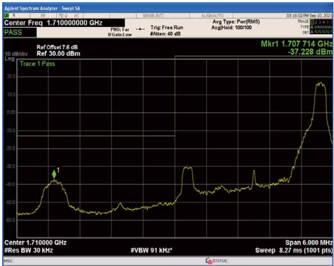
Band4 QPSK BW=3MHz Channel=20385 RB Size=1 Position=#Max
