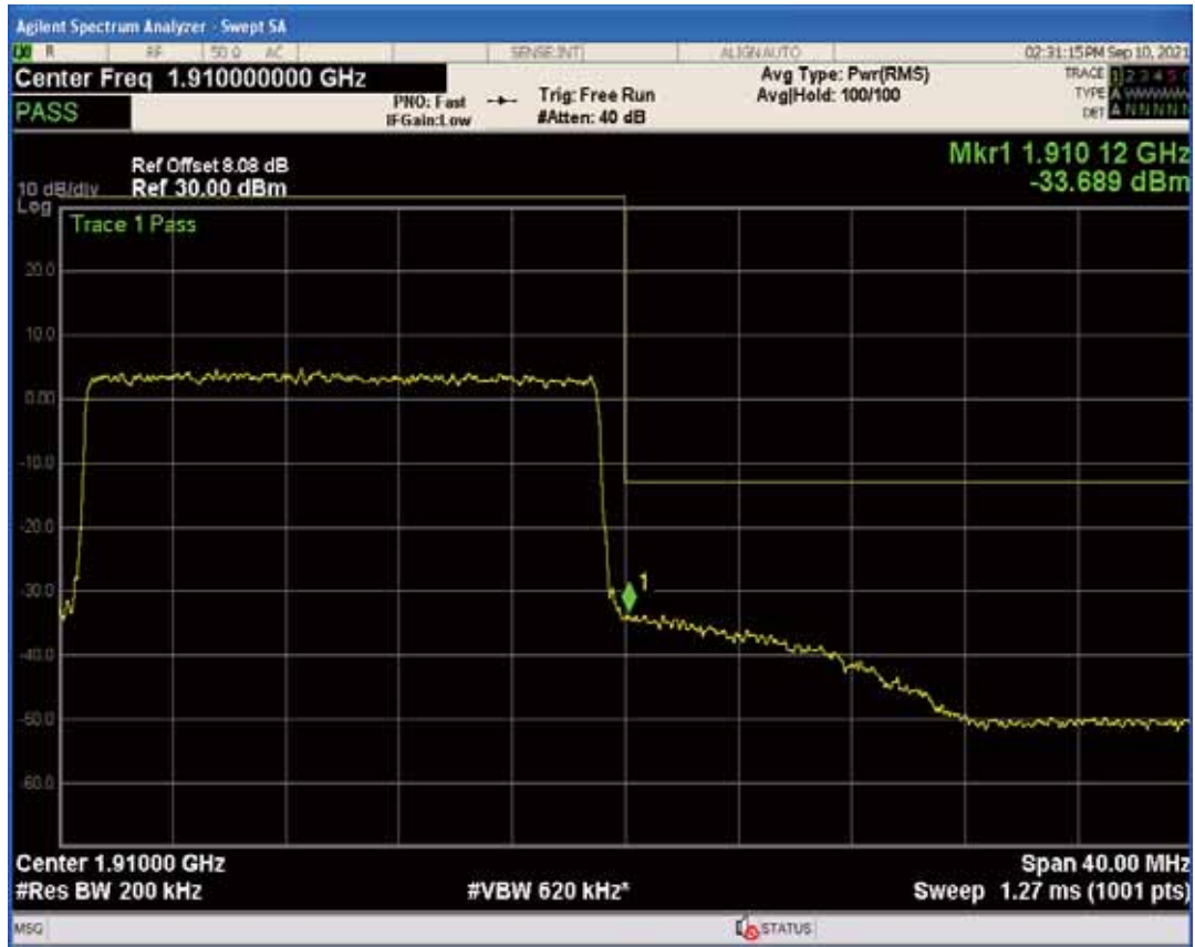
Band4 QPSK BW=1.4MHz Channel=19957 RB Size=1 Position=#0
