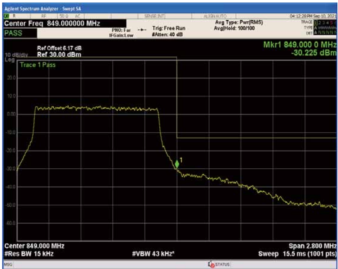
Band5 QPSK BW=3MHz Channel=20415 RB Size=1 Position=#Max
