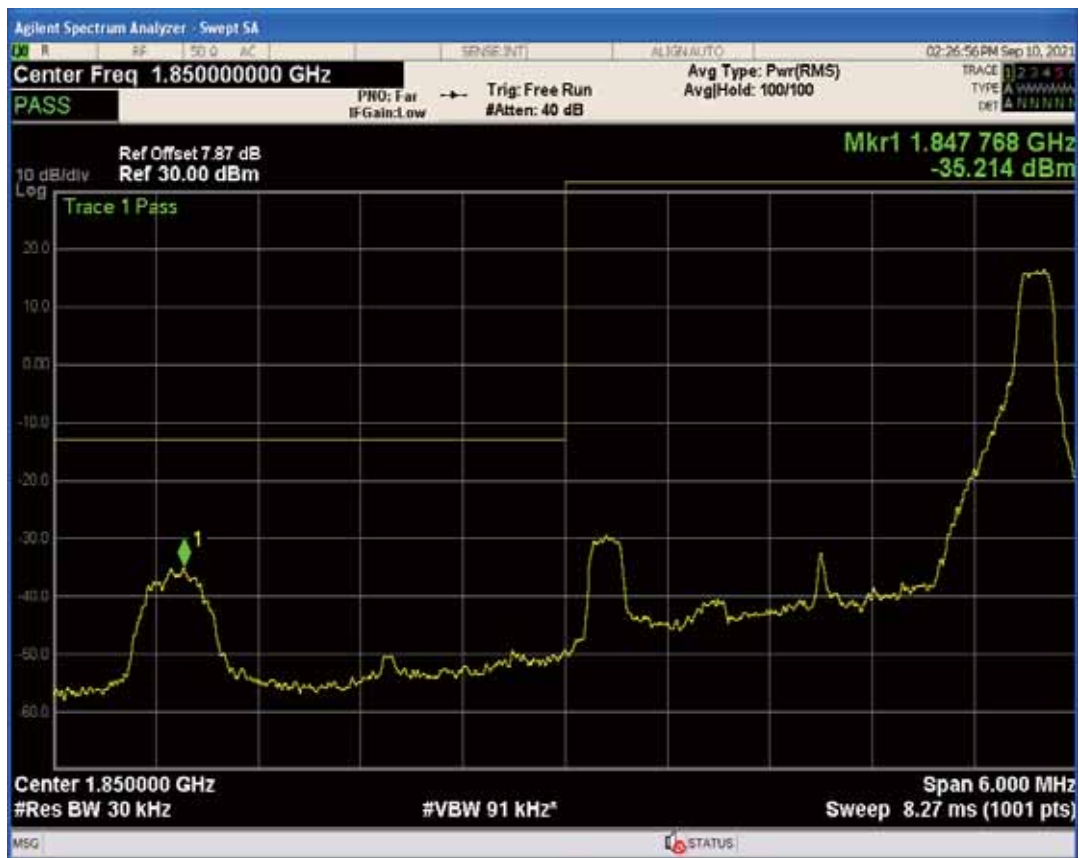
Band2 QAM16 BW=3MHz Channel=18615 RB Size=15 Position=#0
