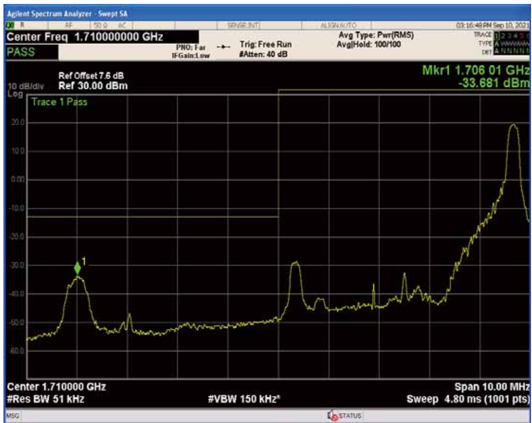
Band4 QPSK BW=5MHz Channel=19975 RB Size=1 Position=#0
