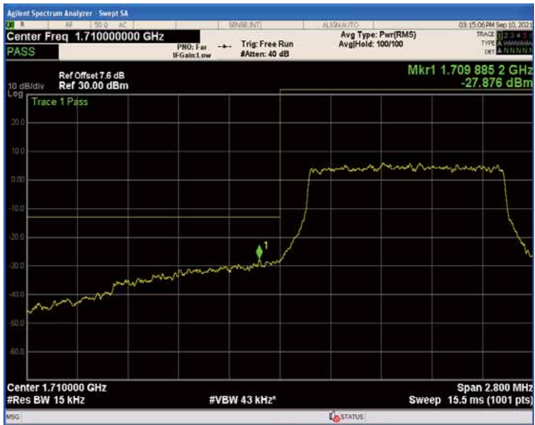
Band4 QPSK BW=1.4MHz Channel=20393 RB Size=1 Position=#0
