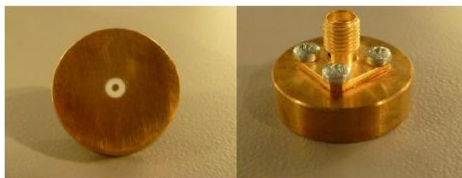
Figure 1 – MVG LIMESAR Dielectric Probe
