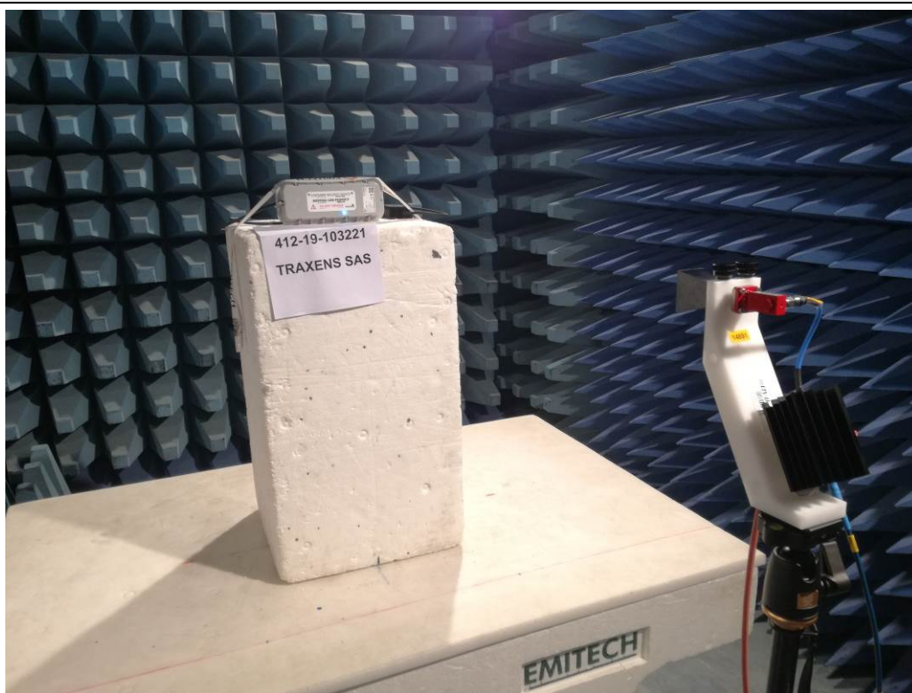
TEST SETUP PHOTO(S) – 18GHz < FREQ
