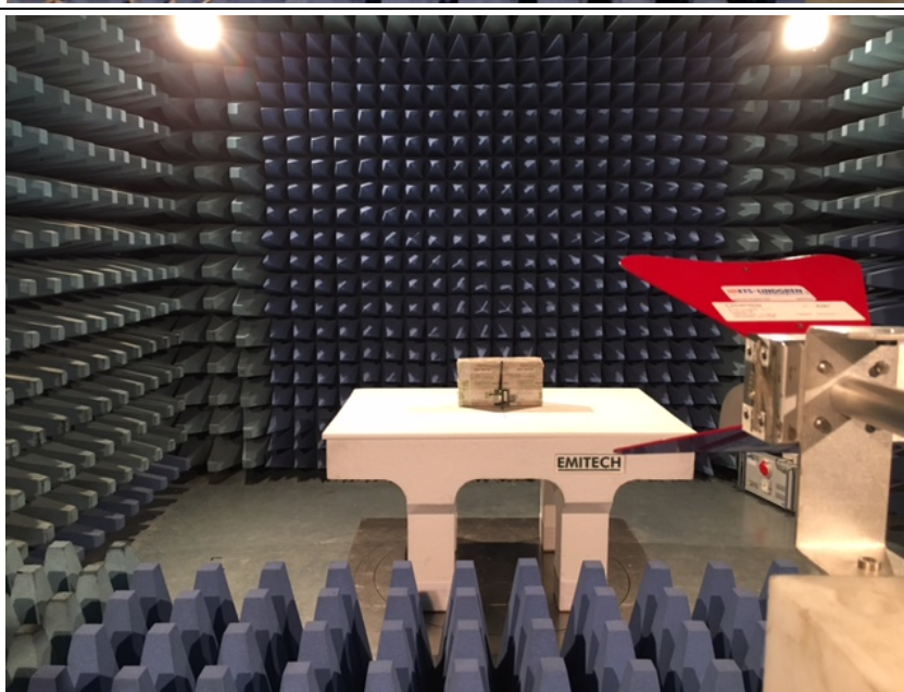
Radiated electric field in anechoic chamber ( f > 1\text{GHz} )
