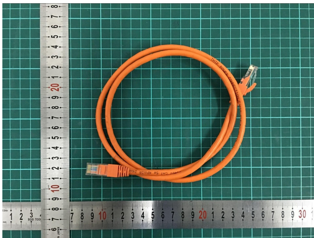
Picture 1-3: Ethernet cables
