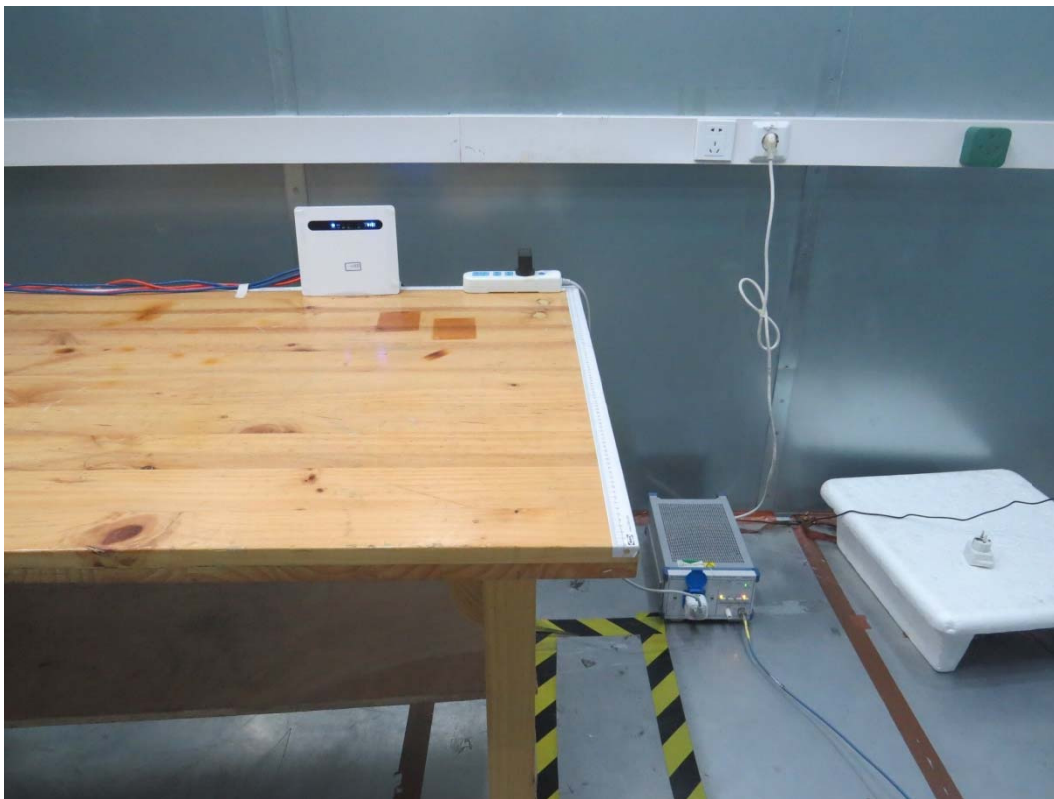
Picture 3 Conducted Emission Test Setup
