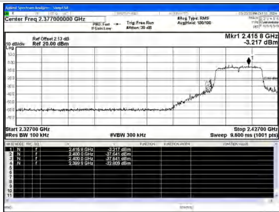
Band Edge NVNT n20 2412MHz Ant1 Emission
