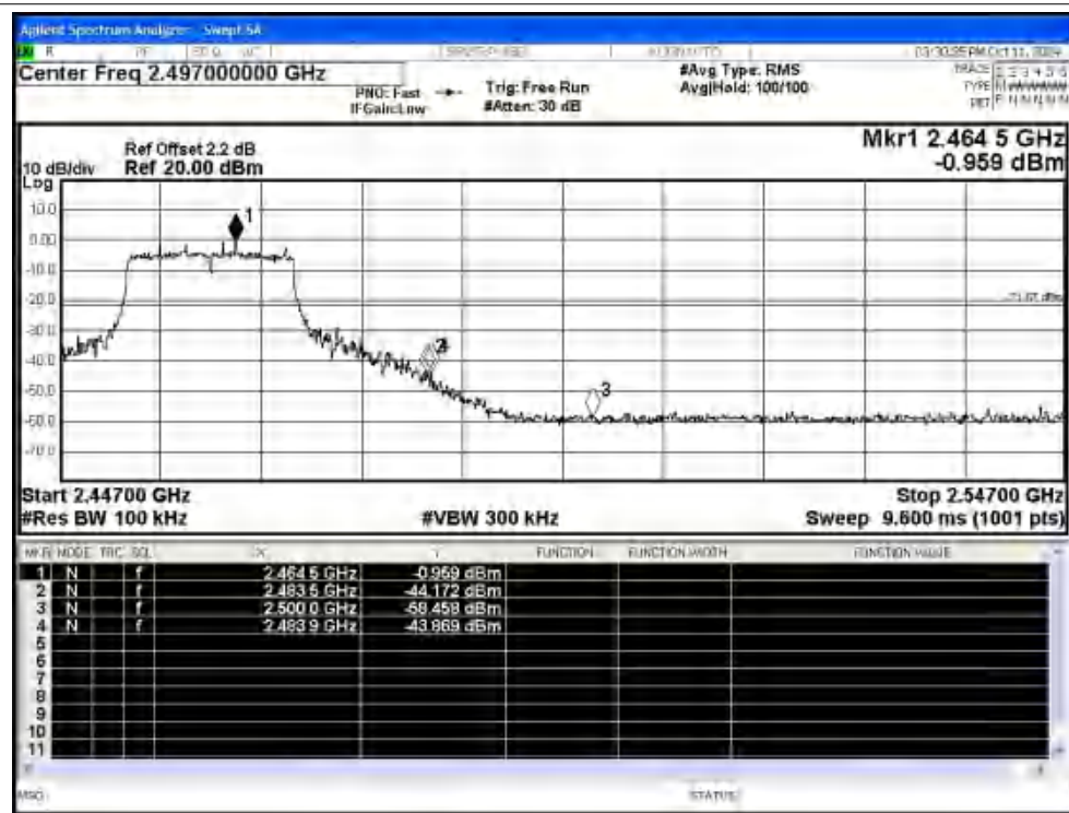
Band Edge NVNT g 2462MHz Ant1 Emission
