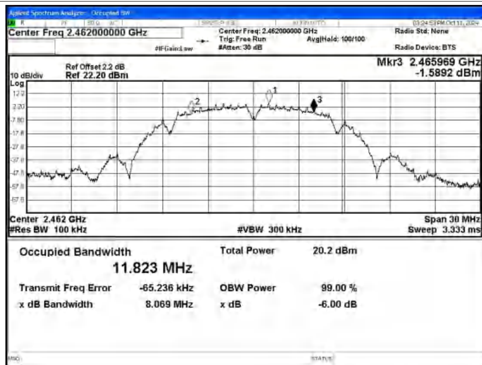
-6dB Bandwidth NVNT g 2412MHz Ant1
