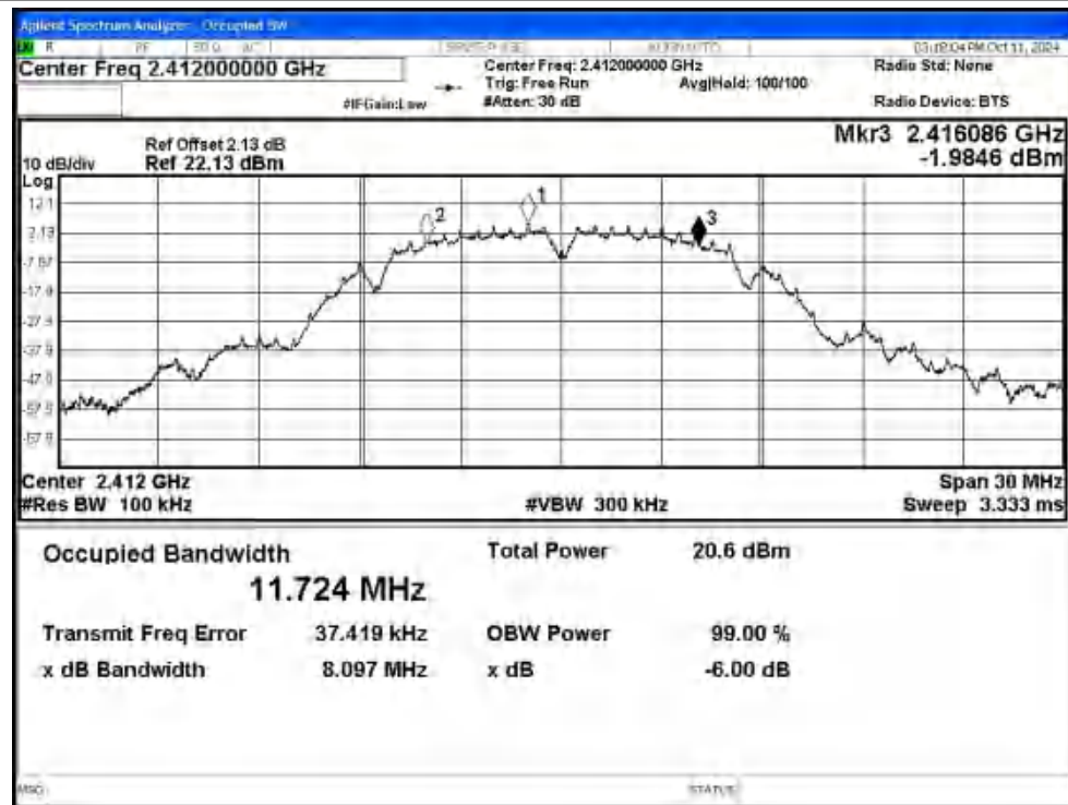
-6dB Bandwidth NVNT b 2437MHz Ant1
