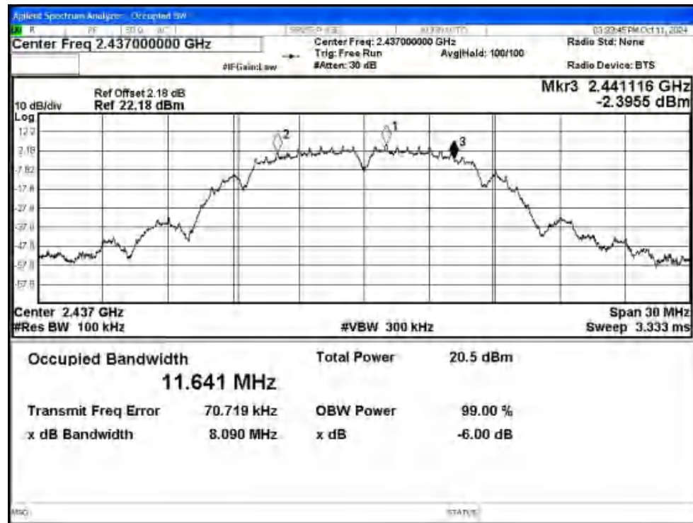
-6dB Bandwidth NVNT b 2437MHz Ant1
