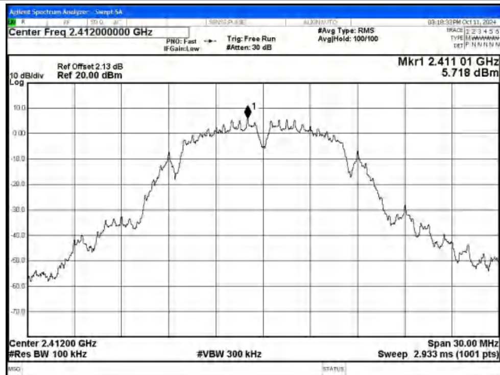
Tx. Spurious NVNT b 2412MHz Ant1 Emission
