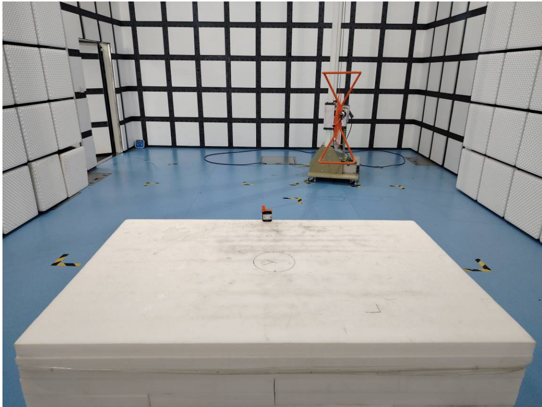
Radiation Emission - Back View (Below 1GHz)
