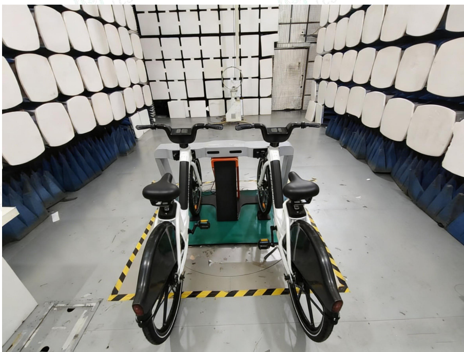
Radiated Emission below 30MHz
