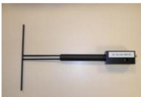
Figure 1 – Satimo COMOSAR Validation Dipole
