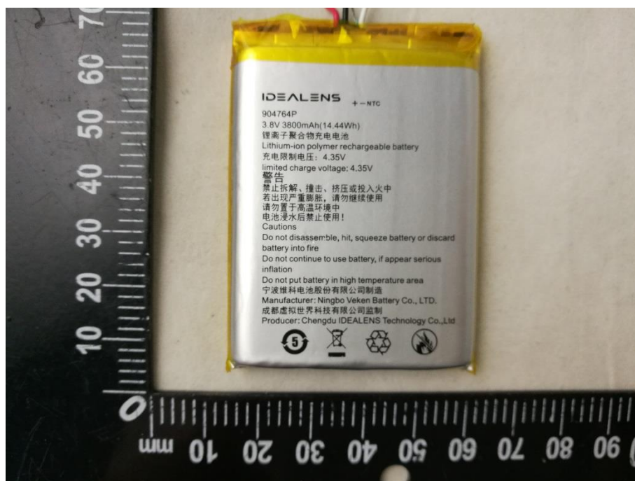
THE BATTERY (FRONT)
