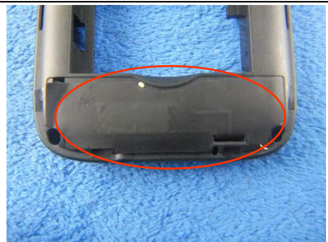
GSM/PCS Antenna View
