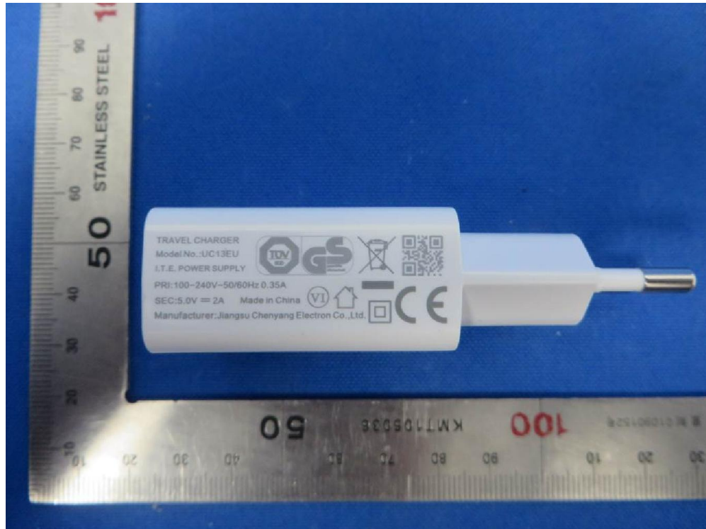
(13) EUT Photo (Adapter, M/N: UC13EU)
