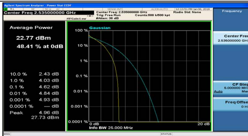
(Channel Bandwidth: 5 MHz)_MCH_QPSK_12RB#6
