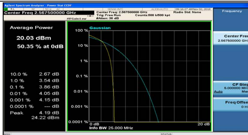
(Channel Bandwidth: 5 MHz)_HCH_16QAM_12RB#6
