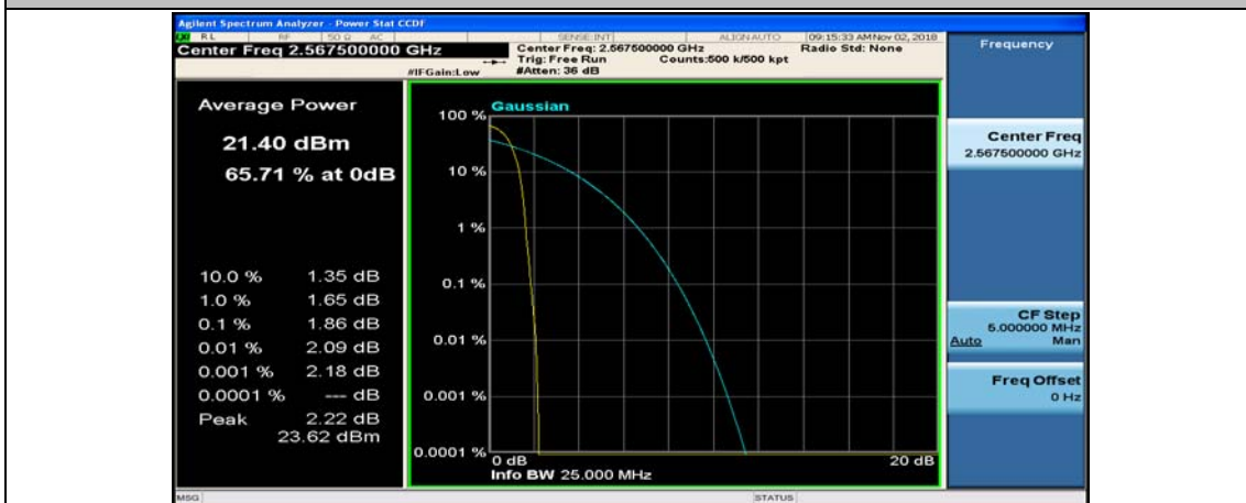
(Channel Bandwidth: 5 MHz)_HCH_QPSK_1RB#12
