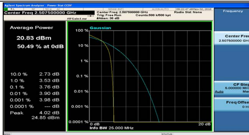
(Channel Bandwidth:15 MHz)_LCH_16QAM_75RB#0
