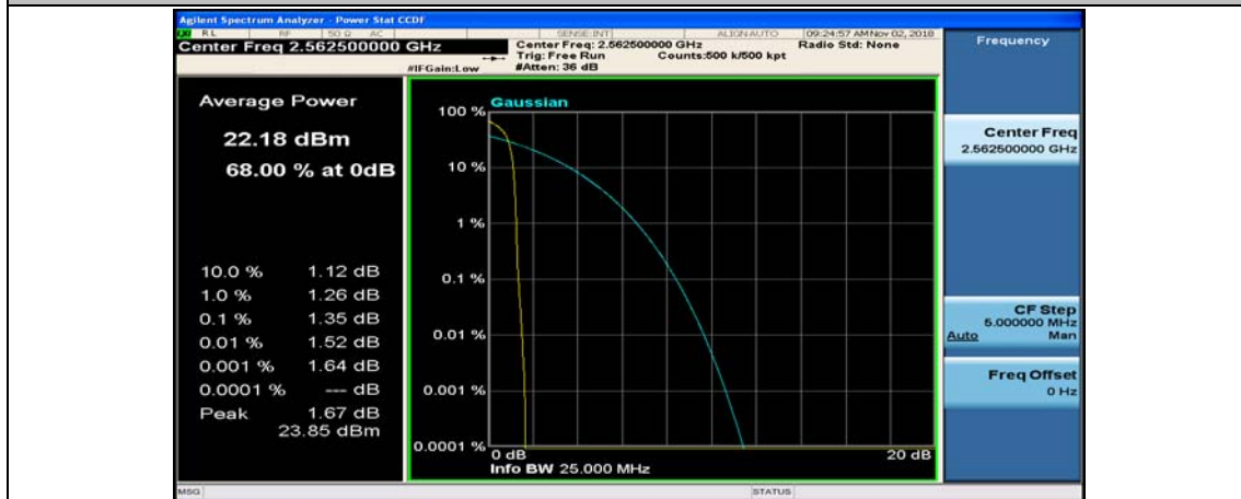
(Channel Bandwidth:15 MHz)_HCH_QPSK_1RB#37
