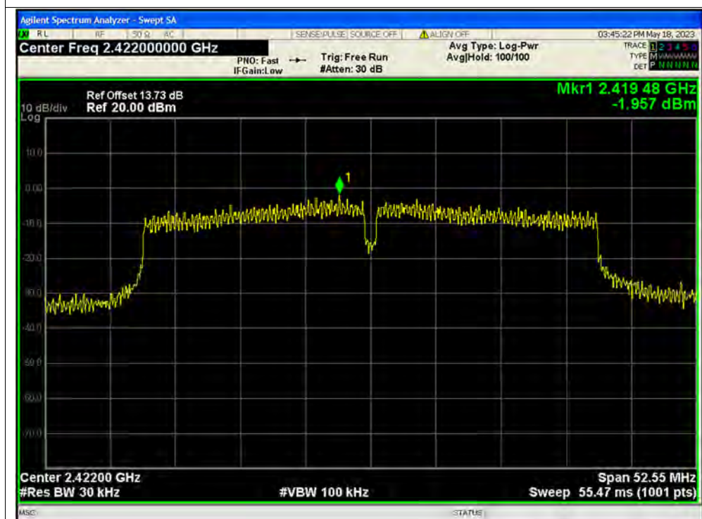
PSD NVNT n40 2422MHz Ant1
